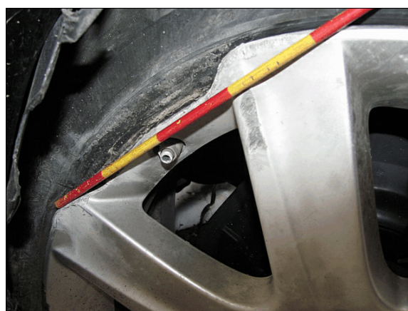
Figure 7: Damage on right front rim from curb impact
