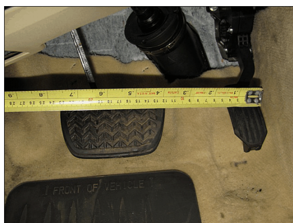
Figure 11: The initial status at inspection of the accelerator pedal, front of the floor mat, and brake pedal of the Lexus
