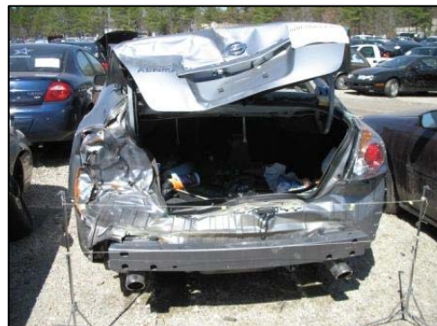
Figure 10. Back plane damage to the Nissan Altima.
