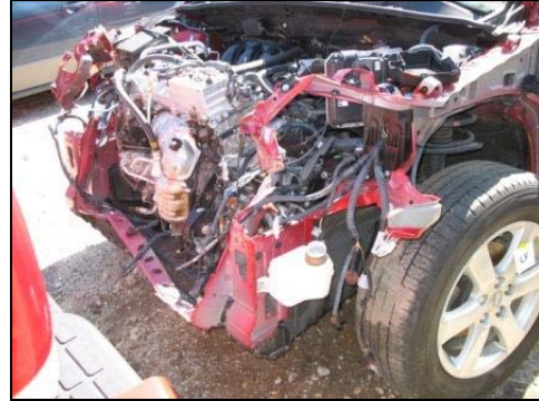
Figure 6. Close-up view of the dismantled damage at the front left area of the Toyota RAV4.
