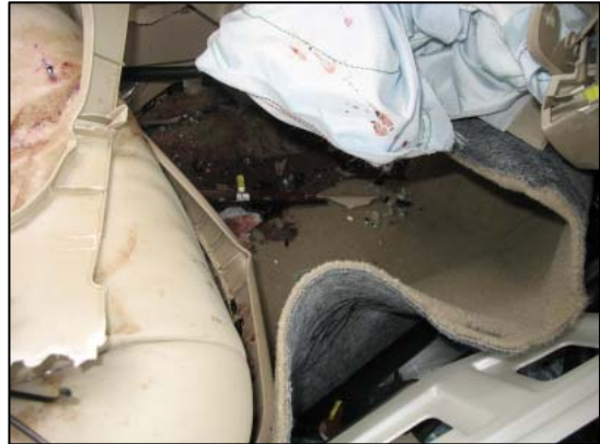
Figure 2: View of the Toyota's driver foot well. No floor mats were located within the foot well.
