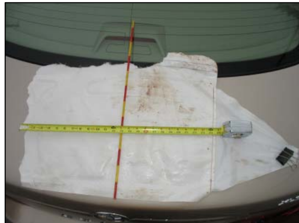
Figure 10: View of the Toyota's left IC and the driver's head contact.
