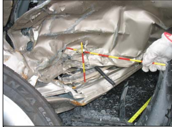
Figure 6: Close-up view of the maximum crush location and the DSD.
