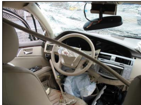
Figure 7: View of the left front interior and the intrusion of the Toyota.
