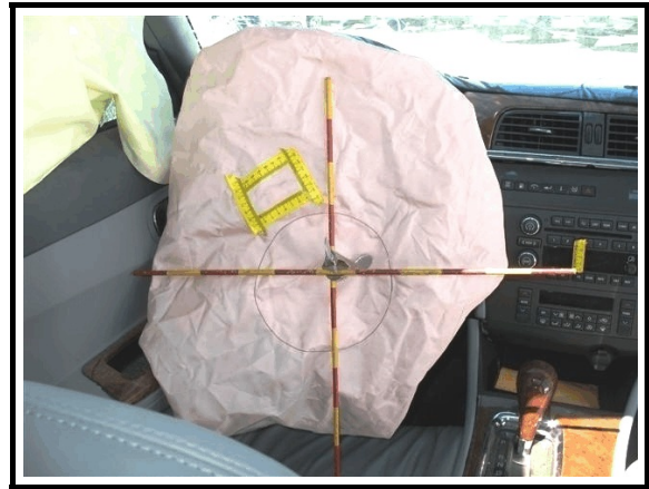
Figure 6. Driver's frontal air bag showing occupant loading to upper left quadrant
