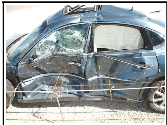
Figure 4. Left side crush documentation showing maximum crush to front left door panel.
