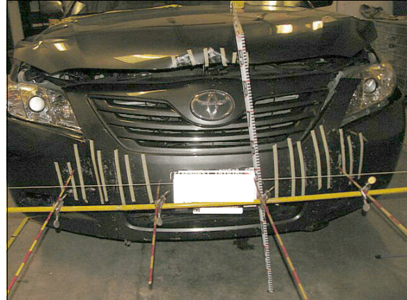
Figure 4: Damage on the front plane of the Toyota from the impact with the building; impressions of the building's fascia are highlighted with tape
