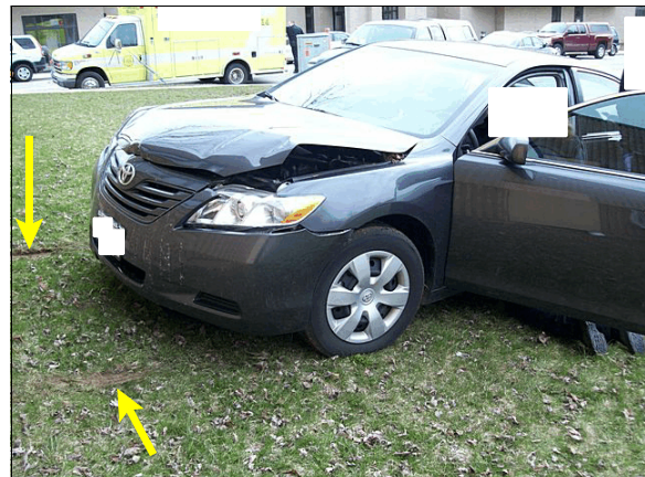
Figure 6: Police photo showing the final rest position of the vehicle; arrows show marks in the grass from spinning front wheels
