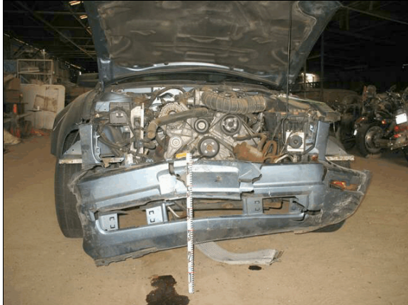
Figure 4: Front of Mustang; vehicle was under repair; bumper fascia placed on end of frame rails; bumper bar had been salvaged
