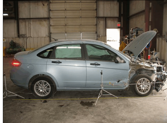
Figure 5: The Focus sustained impact damage on the right fender and right front door
