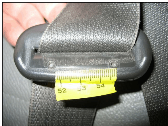
Figure 8: Load abrasion on the driver's latch plate belt guide
