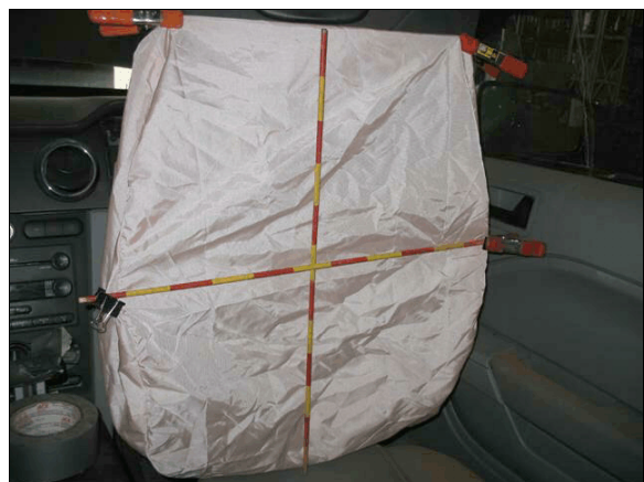
Figure 7: The deployed front passenger's frontal air bag
