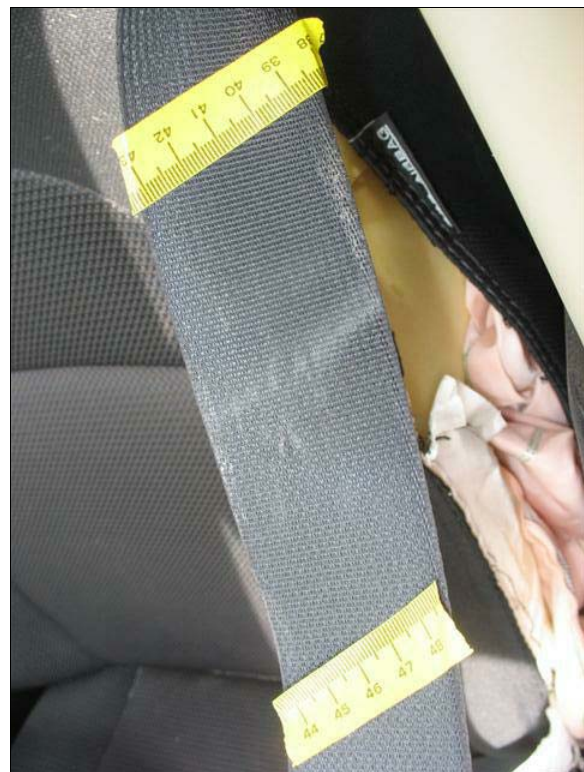
Figure 9: Load marks on the driver's safety belt webbing
