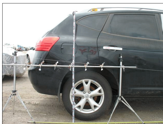
Figure 4: Damage on the right side of the Nissan from the impact with the front of the Lexus
