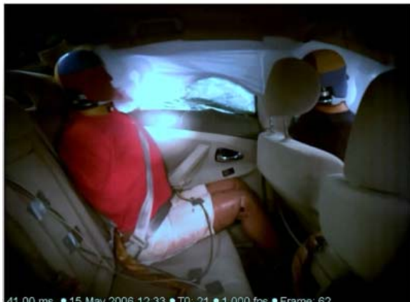
Figure 23: Right interior view of the deploying IC in NHTSA test #5674 at 41 milliseconds post-impact.
