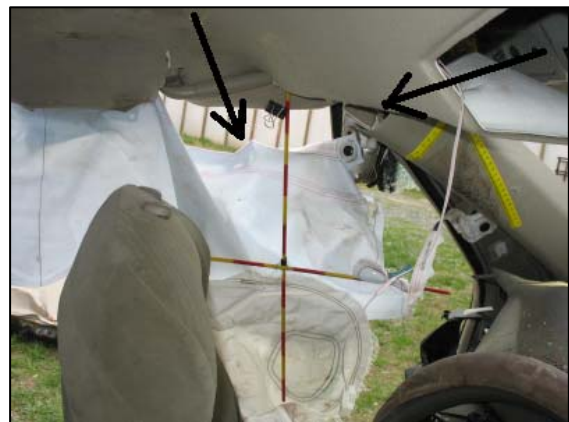
Figure 18: Right lateral view of the deployed left IC and seat-mounted air bag.
