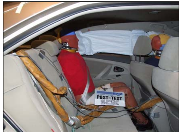
Figure 17: Right interior post-crash test view of a 2007 Toyota Camry, NHTSA test #5674.
