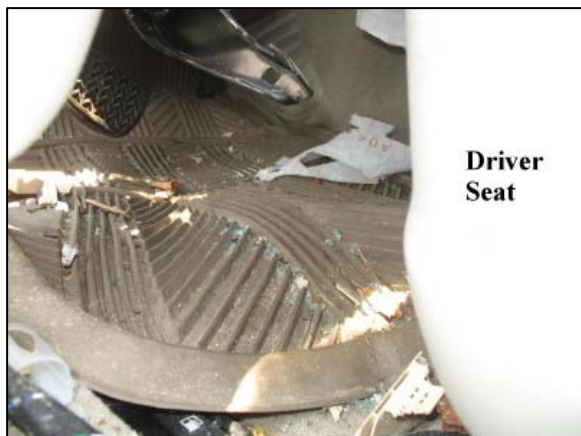
Figure 2: Driver floor area and the aftermarket floor mat.
