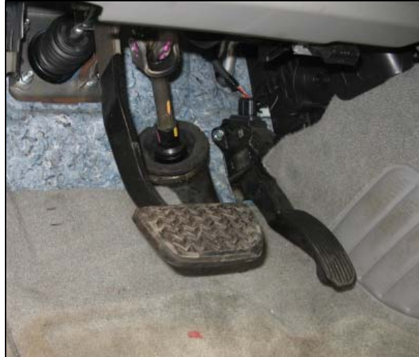
Figure 21: View of the foot controls in an exemplar undamaged 2007 Toyota Camry. Note the angle of the accelerator pedal, as compared to Figure 19.
