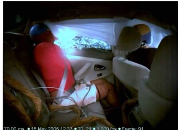
Figure 24: Right interior view of the deploying IC in NHTSA test #5674 at 70 milliseconds post-impact.
