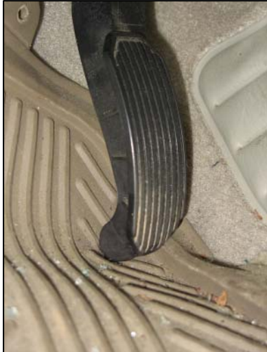
Figure 20: View of the accelerator pedal in contact with the floor mat.
