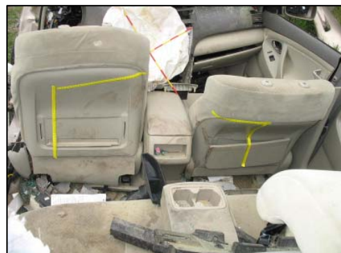
Figure 15: View of the contacts to the front row seat backs
