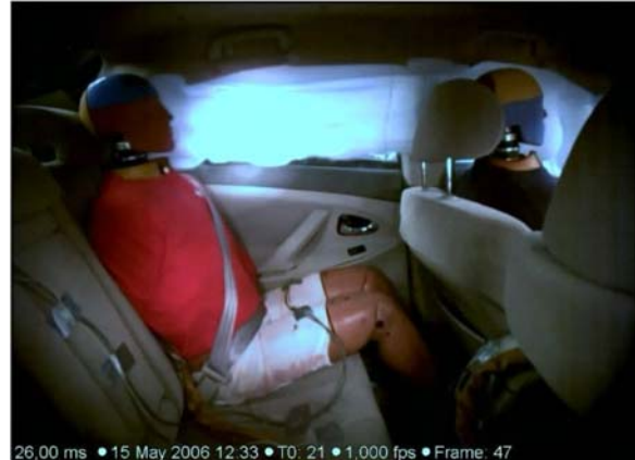
Figure 22: Right interior view of the deploying IC in NHTSA test #5674 at 26 milliseconds post-impact.
