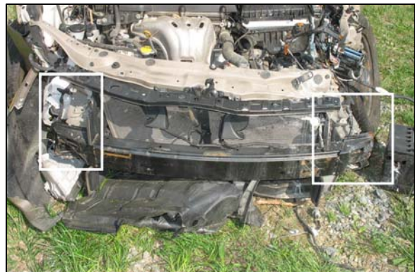
Figure 8: Close-up view of the reinforcement beam.
