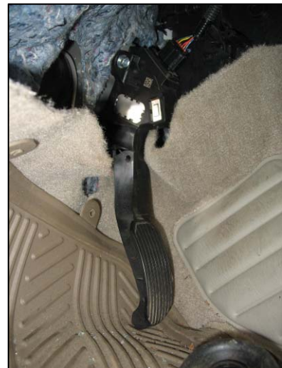
Figure 19: Post-crash position of the Toyota's accelerator pedal.
