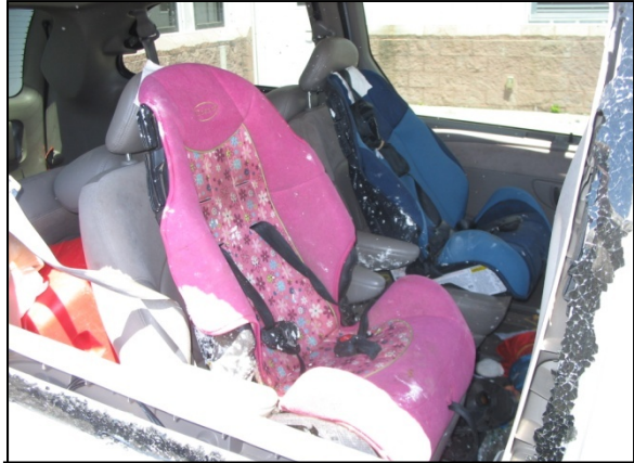
Figure 7: Right interior view of the Chrysler and the reconstructed positions of the CRS's.
