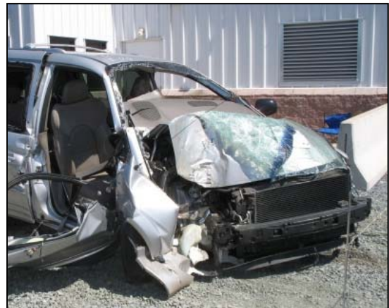
Figure 5: Right side view of the pole impact damage.
