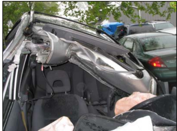
Figure 4: View of the deformed windshield header.
