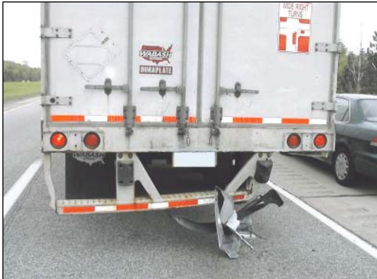
Figure 5: Rear view of the trailer depicting the deformed rear impact guard.
