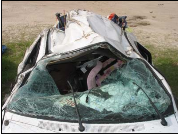
Figure 8: Front view of the roof deformation.
