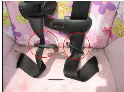
Figure 16: View of the harness straps roped within the buckle clips.
