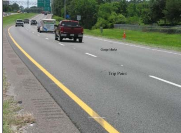
Figure 5: Roll trajectory of the Ford.
