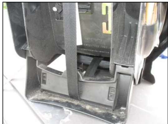
Figure 17: View of the improperly routed adjustment strap.
