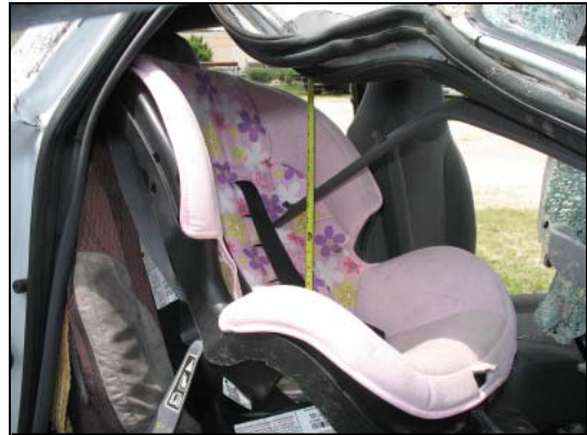
Figure 15: View of the CRS reconstructed into the front right seat position.
