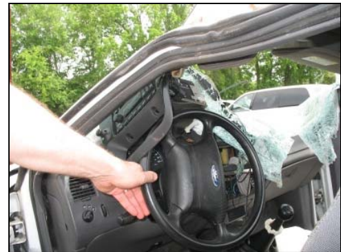
Figure 11: View of the left interior depicting the displaced radio and jammed steering wheel rim.
