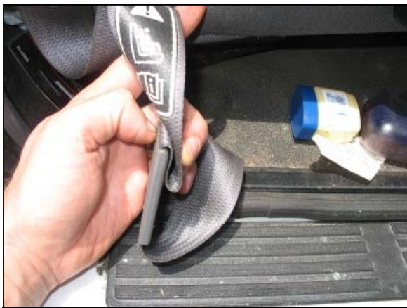
Figure 12: View of the reconstructed pre-crash condition of the EML.
