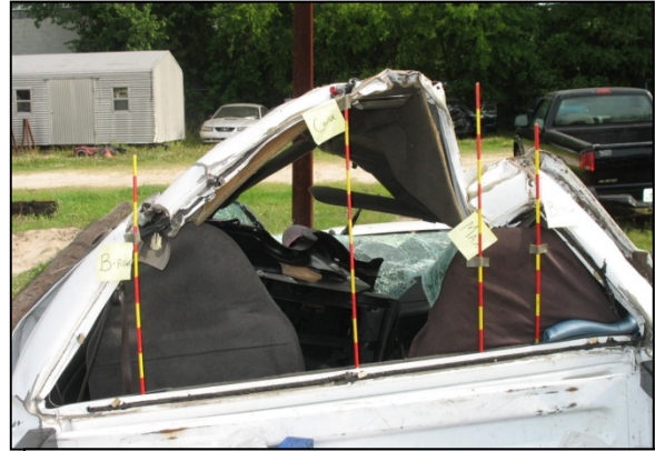
Figure 9: Back view of the roof and backlight header deformation
