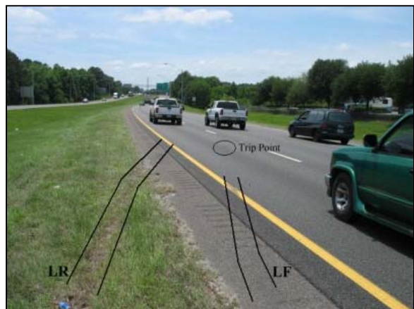
Figure 4: View of the Ford's yaw marks as the vehicle reentered the travel lane.
