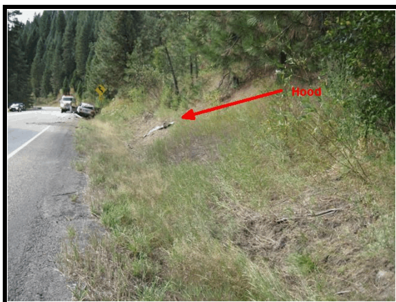
Figure 13. Impact with ground after vault (police photo)
