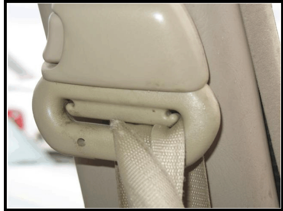
Figure 9. Driver's safety belt webbing at D-ring
