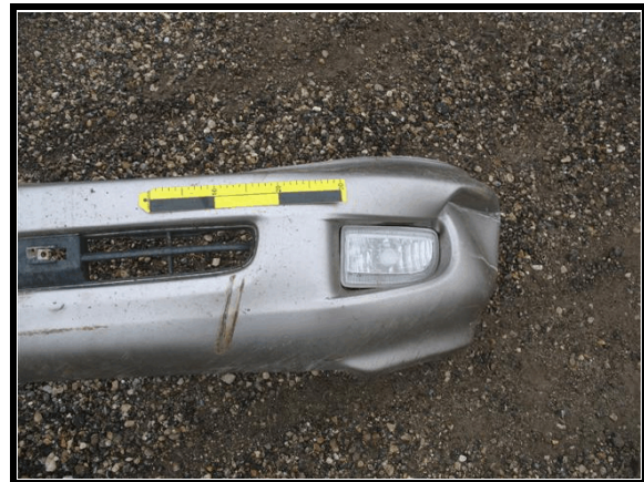
Figure 5. Front bumper damage from impact with snow pole
