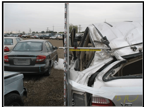
Figure 8. Maximum lateral and vertical crush at left D-pillar
