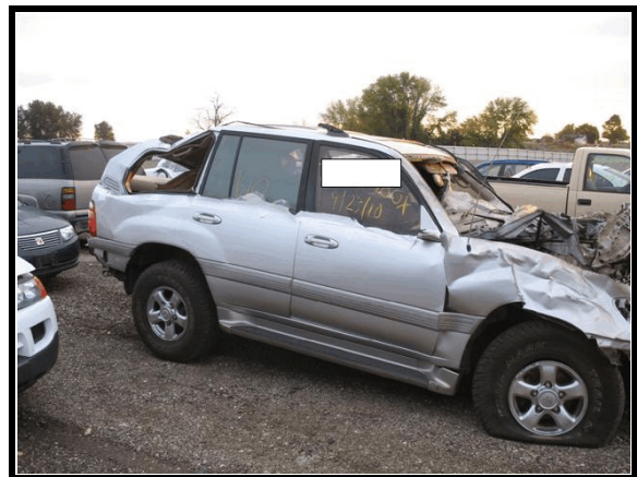
Figure 7. Overview of rollover damage
