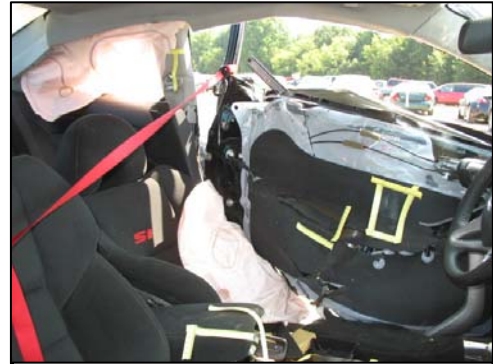
Figure 5: Front left seat compression due to left side intrusion.
