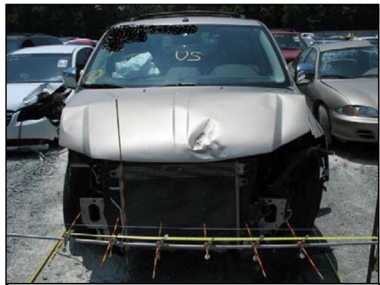
Figure 8: Frontal damage sustained by the Dodge minivan.
