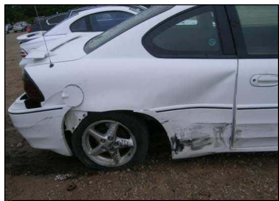
Figure 9: Right side sideswipe damage to the Pontiac.
