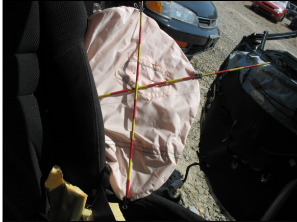
Figure 6: Inboard side of left side air bag.
