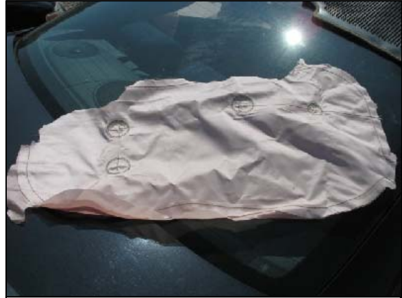
Figure 7: Forward aspect of the IC air bag cut by EMS.
