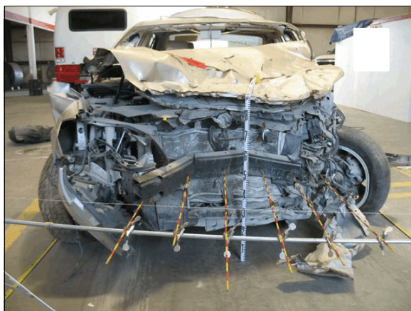
Figure 3: Damage on the front plane of the Toyota from the impact with the back plane of the Infiniti
