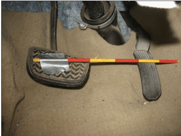
Figure 5: The Toyota's brake and accelerator pedal, each increment on the measurement rod is 5 cm (2 in)
