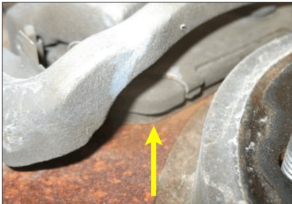
Figure 7: The bottom portion of the outside brake pad (arrow) on the left front wheel of the Toyota
