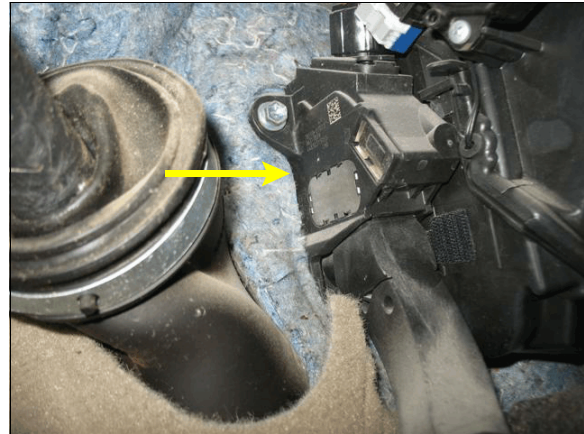
Figure 6: The CTS accelerator pedal mechanism housing (arrow)
