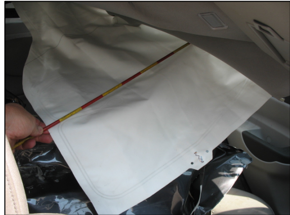
Figure 7: View of the forward interior aspect of the Hyundai’s left IC air bag.
