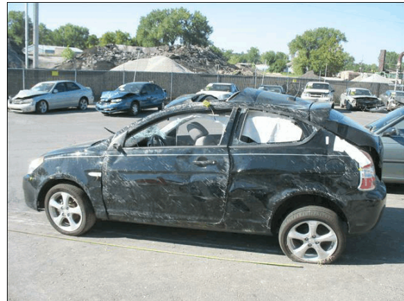
Figure 5: Damage from the rollover on the left side and top planes of the Hyundai
