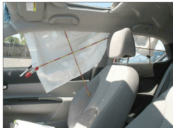
Figure 8: The partially deployed right IC air bag
