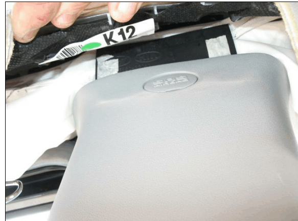
Figure 7: The Hyundai's right IC air bag was entrapped at the top of the right B-pillar and did not fully deploy
