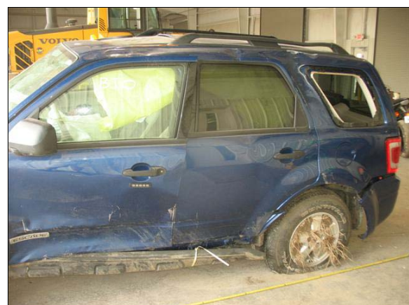
Figure 6: Damage from the rollover on the left plane of the Ford
