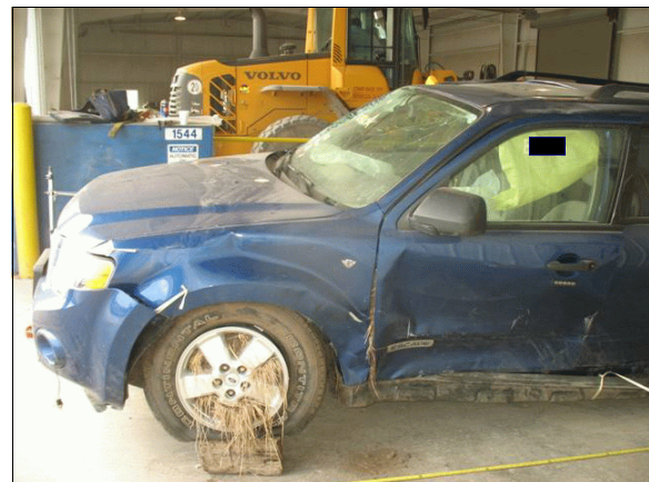
Figure 5: Damage from the rollover on the left plane of the Ford
