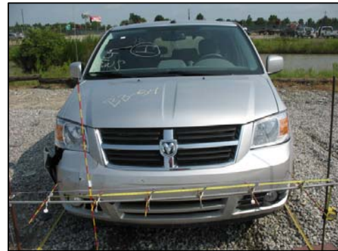
Figure 4: Event 2 damage to the front plane of the 2010 Dodge.
