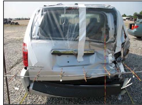
Figure 3: Initial impact damage to the rear of the 2010 Dodge.
