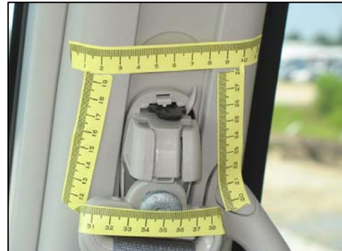
Figure 8: Damage to the front right safety belt height adjustment.
