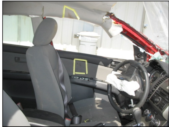
Figure 4: Left side occupant contact evidence in the Nissan.
