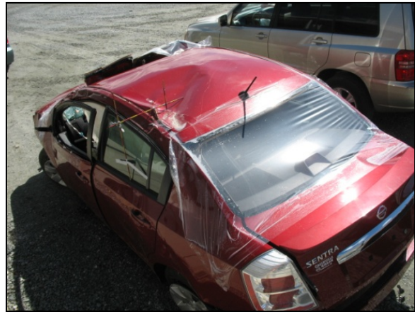
Figure 3: Rollover damage to the top plane of the Nissan.
