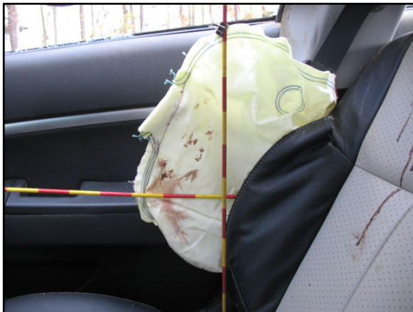
Figure 5: Inboard side of the right side impact air bag.
