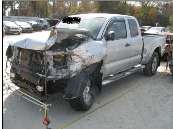
Figure 8: Frontal and left side damage to the
