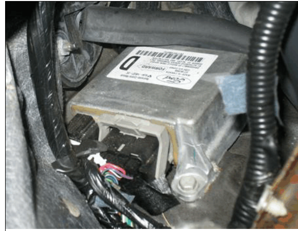
Figure 8: The condition of the Ford's ACM prior to removal from the vehicle
