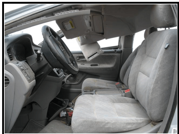
Figure 7. Overview of front row roof intrusion
