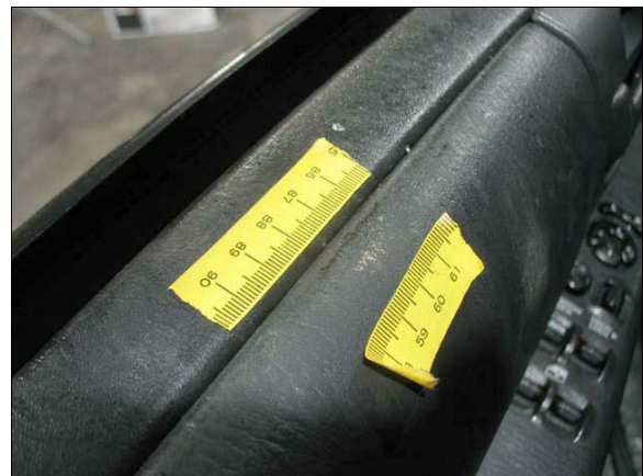
Figure 5: Scuff on beltline of driver's door of the Dodge
