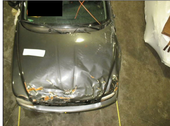
Figure 3: Rollover and cable guardrail damage to hood/left fender of the Dodge
