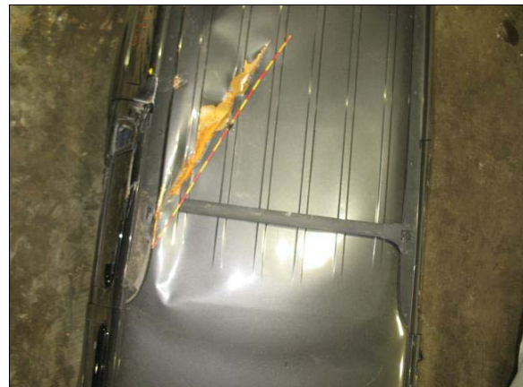
Figure 4: Damage from cable guardrail on roof of the Dodge
