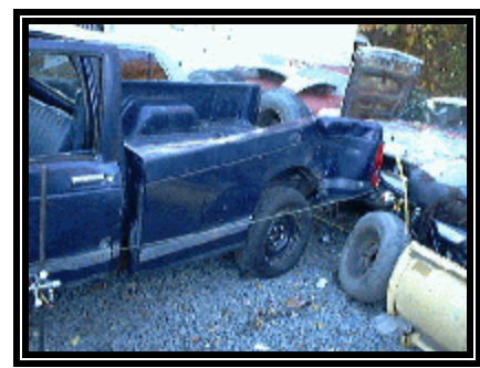
Figure 5: Left side damage of the Chevrolet S-10 pick-up.
