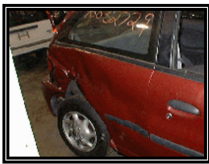
Figure 4: Right side damage of the Geo Metro.
