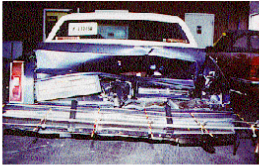
Figure 5. View of the damaged back plane of the Oldsmobile.
