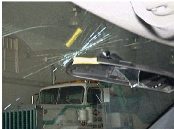
Figure 9. Displaced and damaged rear view mirror and fractured windshield.
