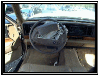
Figure 6: Deformed driver air bag module.
