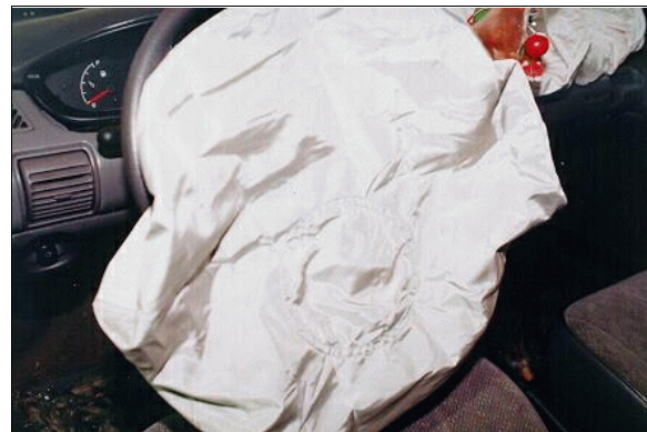
Figure 9: Case vehicle's deployed driver air bag showing no obvious evidence of occupant contact (case photo #19)
