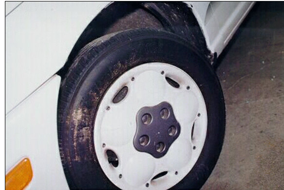
Figure 8: Close-up of scuffs and scrapes on case vehicle's inward rotated left front wheel from north curb impact (case photo #16)
