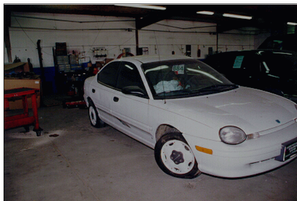
Figure 5: Case vehicle's front and right side showing no obvious contact damage inward rotation of right front tire (case photo #11)
