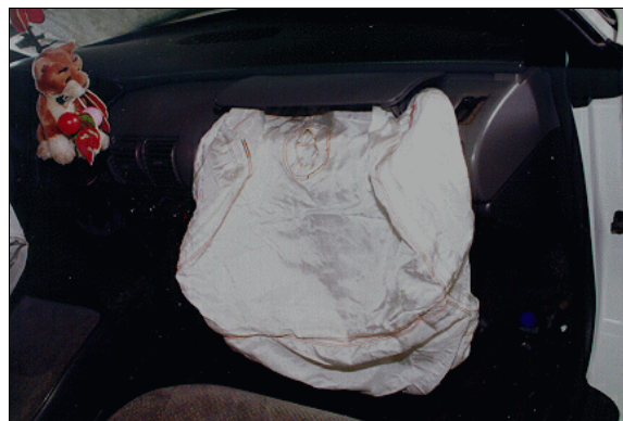
Figure 10: Case vehicle's deployed front right passenger air bag (case photo #22)
