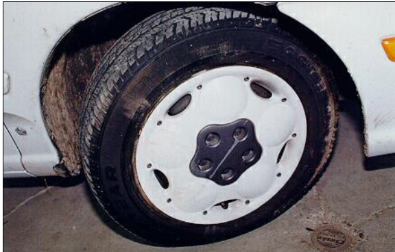
Figure 7: Close-up of scuff marks on case vehicle's inward rotated right front tire (case photo #14)
