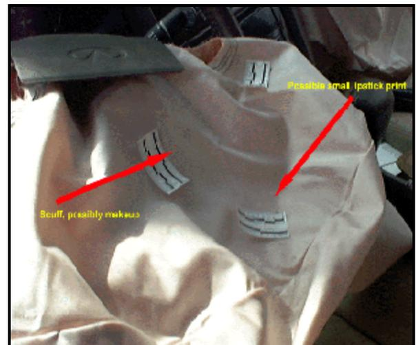
Figure 5. Back side of driver airbag
