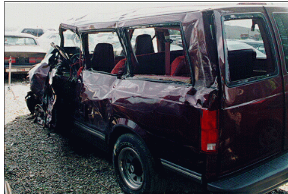
Figure 12: Case vehicle's left side viewed from left of back showing contact damage to all four pillars from impact with rearward protruding corner of Mack's dump truck bed (case photo #26)
