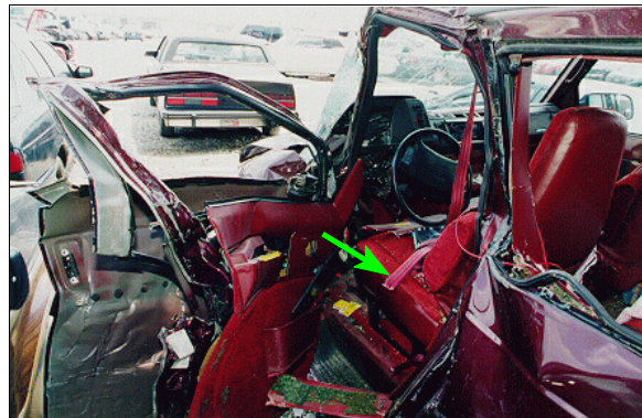
Figure 13: Closer-up view of direct damage to case vehicle's driver door and "A"- and "B"-pillars; Note: intrusion into driver seating area, cut seat belt, and non-deployment of driver's air bag (case photo #38)
