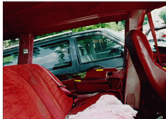
Figure 17: Case vehicle's second seating area showing occupant contact evidence to left side panel and intrusion into second row bench seat, causing serious injuries to second seated left passenger (case photo #47)
