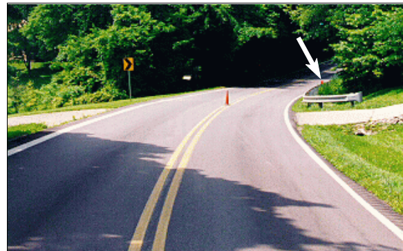
Figure 2: Mack truck's northwestward travel path after re-entering roadway from right (northeast) shoulder; Note: Mack went into a clockwise yaw, crossed the centerline, and struck the case vehicle in the opposing lane (near orange cone on the centerline) before sliding into the guardrail off the right-hand side of the road near the high-lighted (arrow) orange cone (case photo #10)
