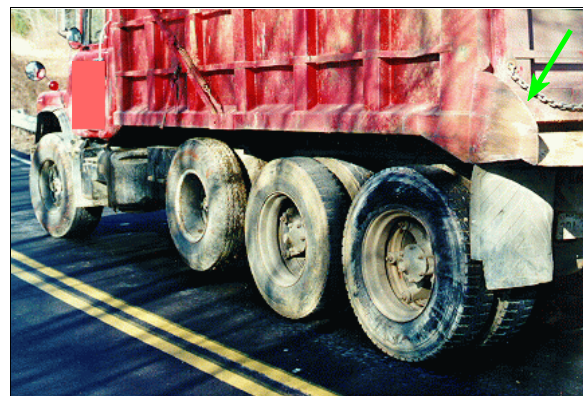
Figure 4: Mack's left side viewed from left of back showing minimal damage (i.e., scuffing) to left rear tandem wheels and scrapes on the rearward protrusion of the left back corner of the dump truck's bed (case photo #52)
