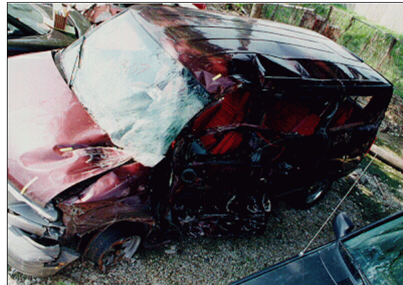
Figure 5: Overhead left view of case vehicle's left side damage from impact with Mack truck's left rear tandem wheels and left back corner of the bed of the dump truck; Note: absence of left front tire and "A"- through "D"-pillar damage (case photo #25)
