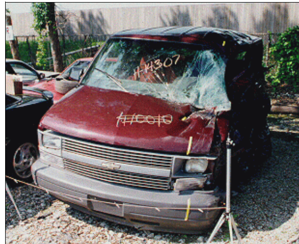
Figure 3: Case vehicle's very narrow front left corner impact; Note: yellow tape on bumper indicates direct damage width from contact with Mack truck's rear tandem wheels and yellow tape on hood shows direct damage width from impact with Mack's dump truck bed (case photo #20)
