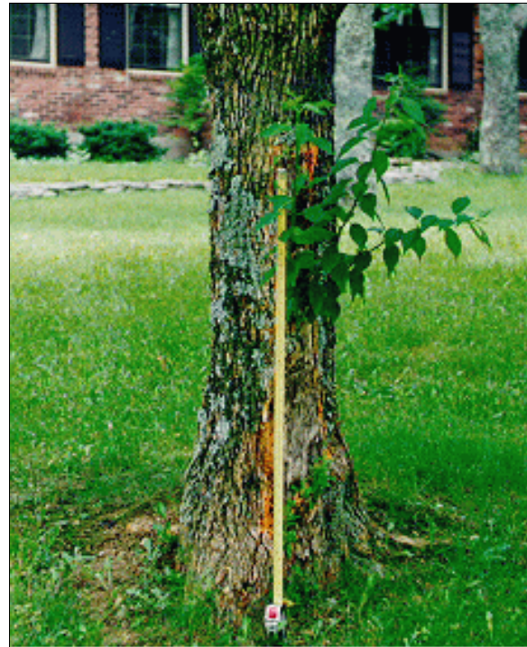
Figure 9: Close-up of yard tree impacted by front left of case vehicle prior to its being redirected south-southeastward to final rest (case photo #08)
