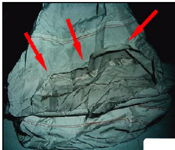
Figure 7. Deployed air bag, arrows mark area where skin tissue was found
