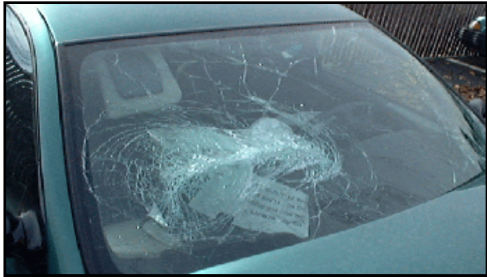
Figure 4. Vehicle exterior, damage to windshield from passenger side air bag
