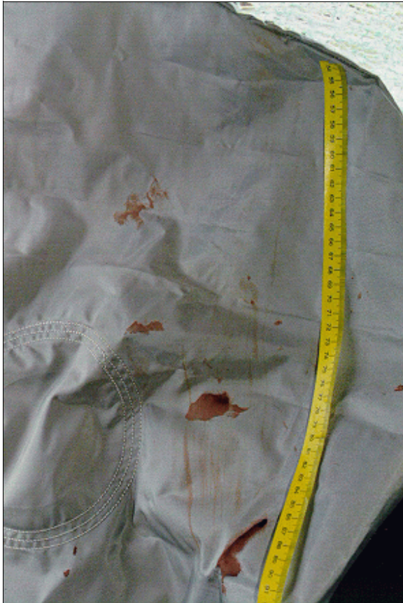
Figure 22: Close-up of skin transfer and blood smear along right side of 1996 GMC Safari's driver air bag to left of yellow tape (case photo #29)
