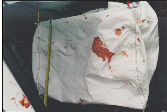
Figure 18: 1996 GMC Safari's front right passenger air bag showing cloth and skin transfer along with blood to front portion (case photo #37)
