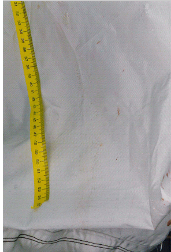
Figure 23: Close-up of skin transfer to top portion of the 1996 GMC Safari's front right passenger air bag from contact by "in-lap" passenger (case photo #41)
