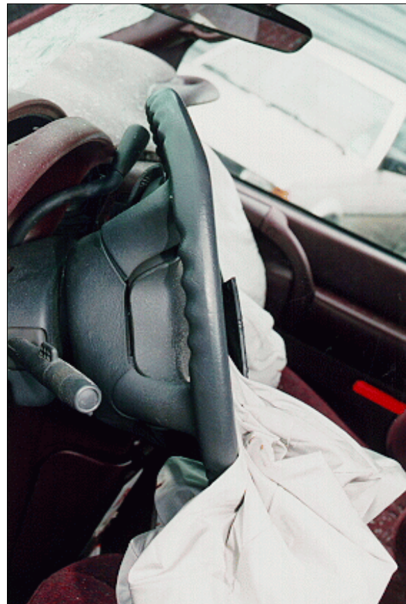
Figure 10: Vertical lateral view of 1996 GMC Safari’s steering wheel rim from left showing deformation to top of rim from loading (case photo #25)
