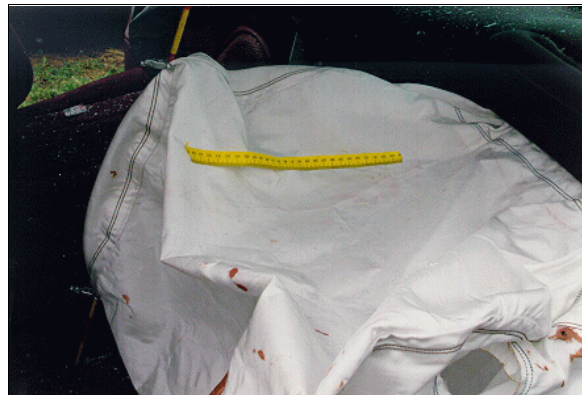
Figure 19: Skin transfer to top portion of 1996 GMC Safari's front right passenger air bag from contact by "in-lap" passenger (case photo #40)
