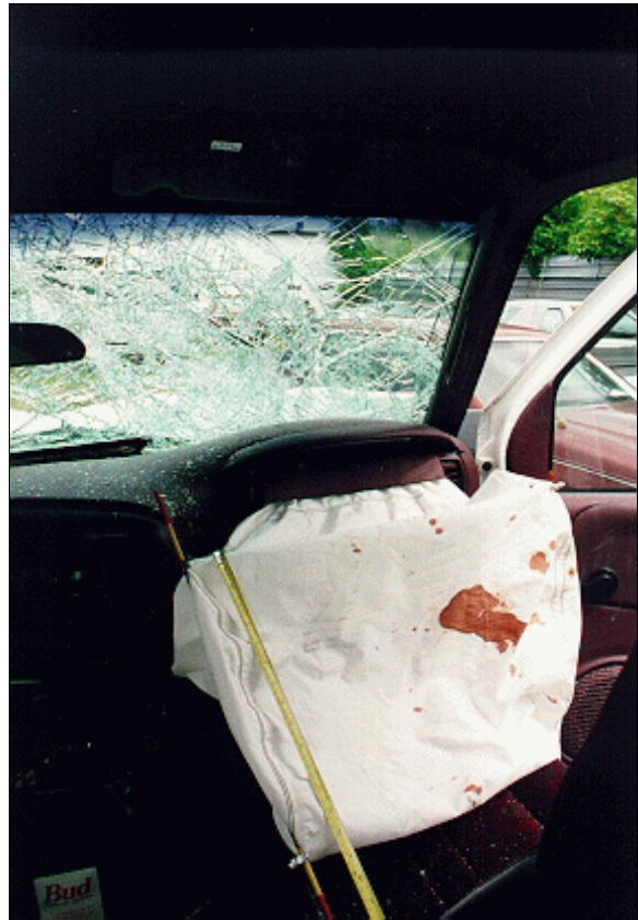
Figure 16: Vertical view of 1996 GMC Safari's deployed front right passenger air bag showing blood evidence on air bag; Note: passenger handle-type grip above top cover flap (case photo #36)
