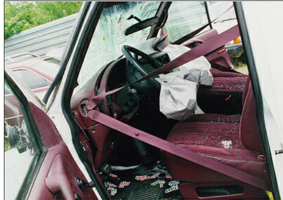
Figure 21: 1996 GMC Safari's outstretched driver seat belt showing no evidence of usage during crash (case photo #32)
