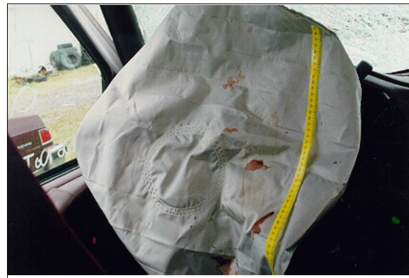
Figure 15: 1996 GMC Safari's deployed driver air bag showing vertical skin transfer (yellow tape) and blood spots on right side of bag (case photo #28)
