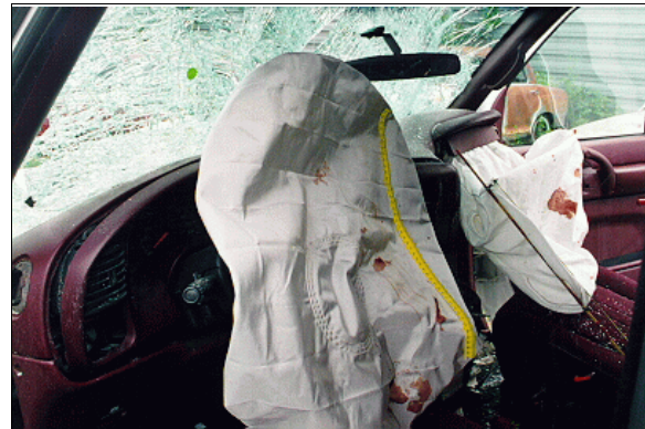
Figure 8: 1996 GMC Safari’s deployed driver and front right passenger air bags; Note: blood on both air bags, contact evidence on windshield, and distorted rearview mirror (case photo #26)
