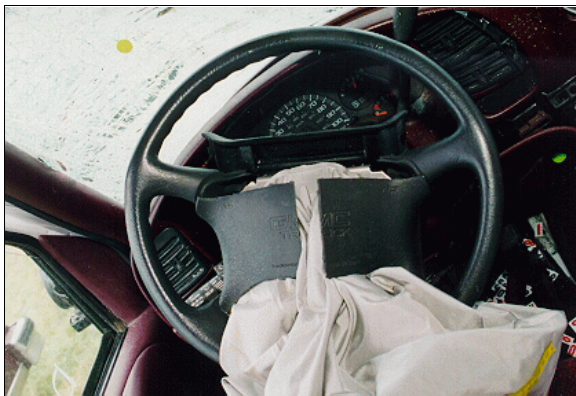
Figure 14: 1996 GMC Safari driver air bag module's three cover flaps (i.e., top, left, and right) showing no occupant contact evidence (case photo #24)
