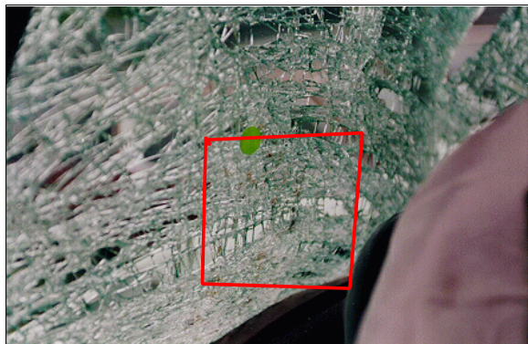
Figure 9: Close-up of interior surface of 1996 GMC Safari’s left windshield showing black plastic transfer from steering wheel rim contact and possible skin transfer from driver’s hand contact (case photo #30)
