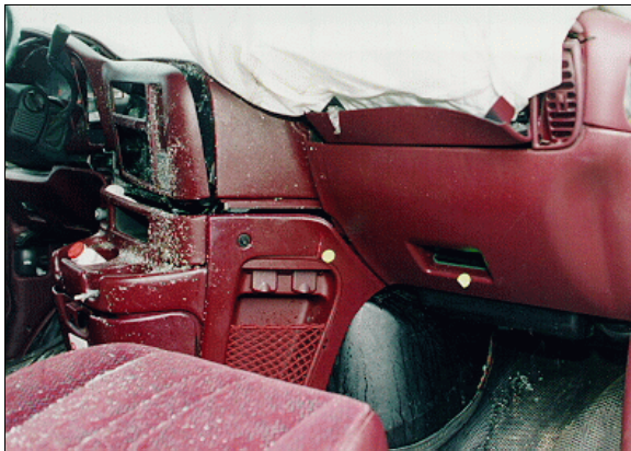
Figure 11: Contact evidence on 1996 GMC Safari's right knee bolster and right side of center instrument panel (case photo #34)
