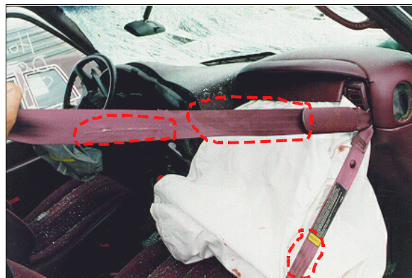
Figure 20: 1996 GMC Safari's front right seat belt showing blood on and stretching to webbing which indicates usage (although improper) during crash (case photo #44)
