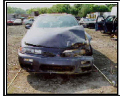
Figure 1. Frontal damage to the Mitsubishi Galant.
