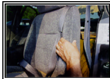
Figure 11. Cut shoulder belt webbing.
