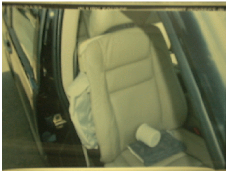
2. View of the deployed passenger side Sipsbag and the separated stitching on the outboard and superior aspects of the right front seat back.
