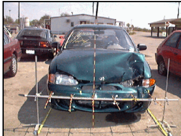
Figure 4: Case vehicle’s front with contour gauge present showing damage from impact with vehicle #2; Note: vehicle #2’s front right bumper corner impacted case vehicle’s front left (case photo #11)
