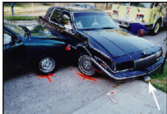
Figure 3: On-scene view of case vehicle (left) and vehicle #2 (right) at final rest; Note: struck brick landscape edging underneath vehicle #2's front bumper (case photo #54)
