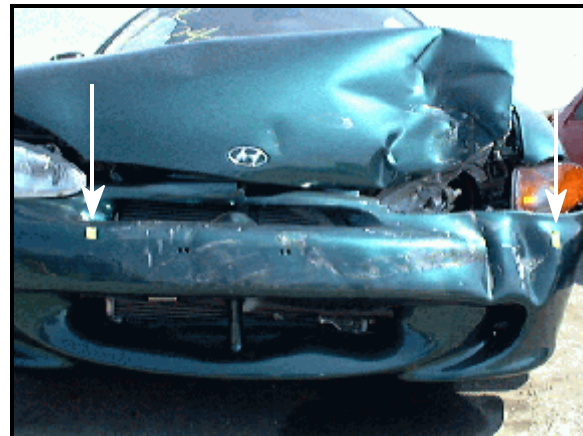
Figure 5: Close-up of direct damage (between yellow tape) to case vehicle’s front bumper and left hood and corner area (case photo #22)
