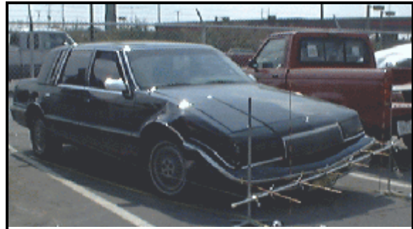
Figure 13: Vehicle #2's damaged front right corner with contour gauge present viewed from right of front (case photo #46)
