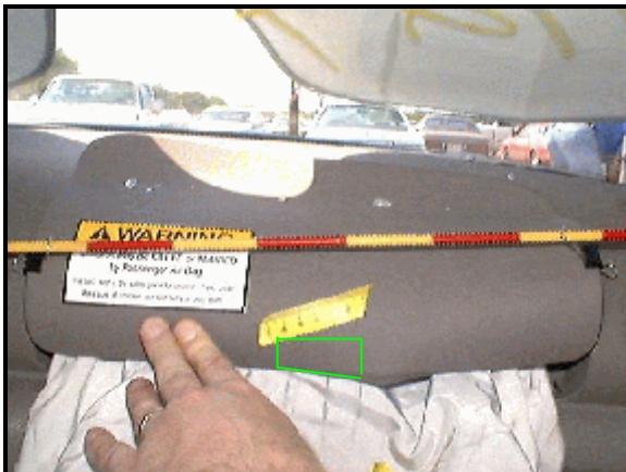
Figure 9: Suspected oil smudge on case vehicle's front right air bag module's cover flap (case photo #34)
