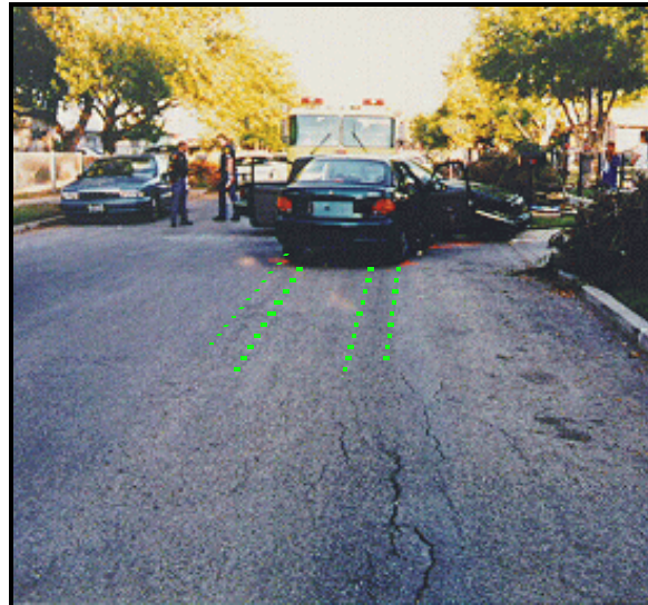
Figure 2: On-scene view of case vehicle and vehicle #2 at final rest positions; Note: highlighted faint tire scrub marks leading to case vehicle's final rest position (case photo #53)
