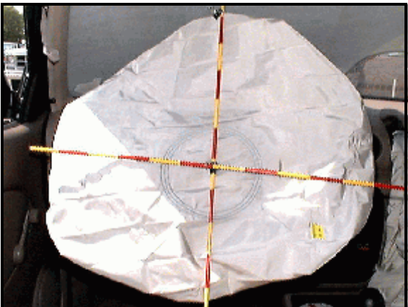
Figure 7: Case vehicle's deployed driver air bag showing area (yellow tape) of mascara transfer near 11 o'clock position; Note: steering wheel has been rotated clockwise (case photo #29)
