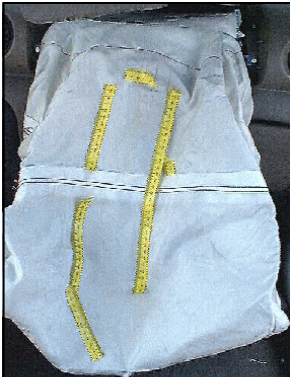
Figure 11: Overhead view of skin transfer to top portion of case vehicle's front right air bag from contact with front right passenger's neck/chin (case photo #37)
