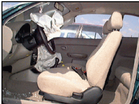
Figure 6: On-scene view of case vehicle's front seating area showing deployed front air bags and close proximity of seats to air bags (case photo #23)
