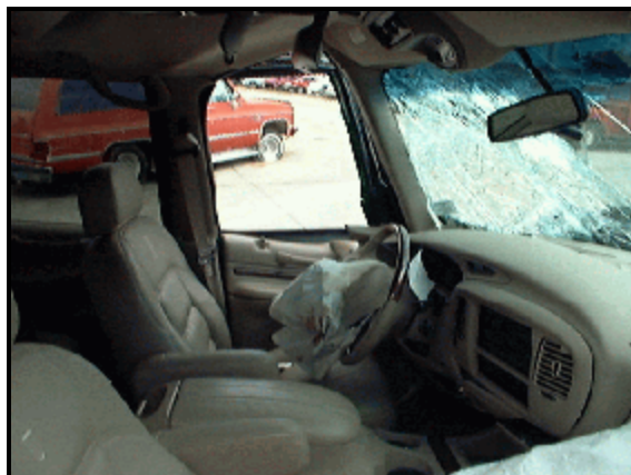
Figure 5: Lincoln's front seating area from right showing deployed front air bags and longitudinal intrusion to driver's seating area from left "A"-pillar and left and center instrument panels (case photo #05)
