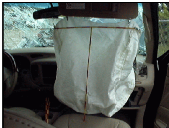
Figure 8: Lincoln's deployed front right passenger air bag showing no occupant contact evidence (case photo #12)
