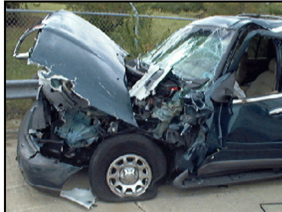
Figure 2: Lincoln's very narrow front left damage viewed from left front; Note: direct damage extends to just short of left "A"-pillar, left "A"-pillar is pushed backwards, and left front tire is deflated and restricted (case photo #02)
