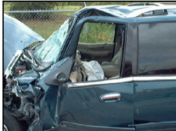
Figure 3: Close-up of Lincoln's driver door area showing narrow frontal impact's penetration along left side, rearward displacement of left "A"-pillar, left roof buckling, and jammed driver's door (case photo #03)
