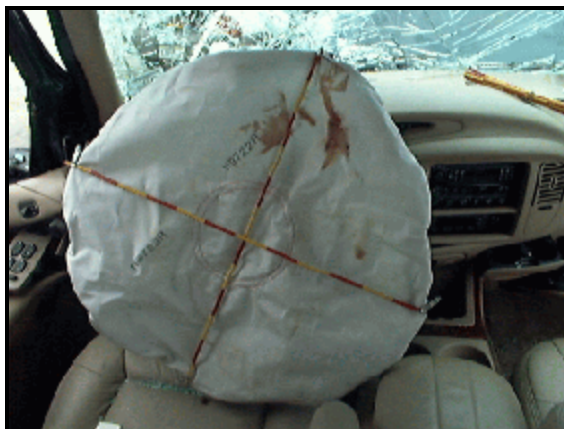
Figure 7: Lincoln's deployed driver air bag showing blood evidence, primarily at 12 o'clock position (case photo #08)
