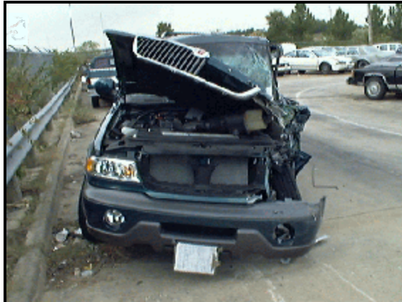
Figure 1: Lincoln's very narrow front left impact viewed from front; Note: Lincoln's front left bumper underrode right front bumper corner of Ford truck-tractor (case photo #01)
