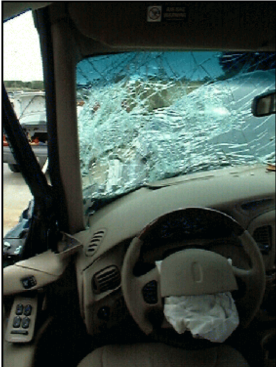
Figure 9: Vertical view of Lincoln's driver seating area showing crash induced damage to windshield's glazing, intrusion from left "A"-pillar and instrument panel, and driver air bag module's top cover flap which was without evidence of contact (case photo #17)
