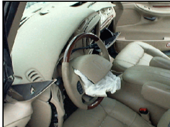
Figure 6: Lincoln's front seating area from left showing longitudinal intrusion to driver's seating area from left and center instrument panels and likely position of driver's seat (case photo #06)
