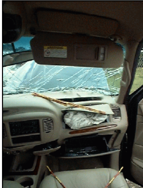
Figure 10: Vertical view of Lincoln's front right passenger seating area showing front right passenger air bag module's cover flap and folded, deployed air bag (case photo #19)
