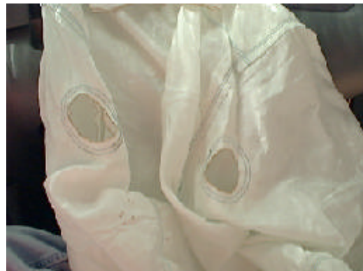
Figure 11 - View of the air bag vent ports along the inboard/outboard side panels of the front right air bag
