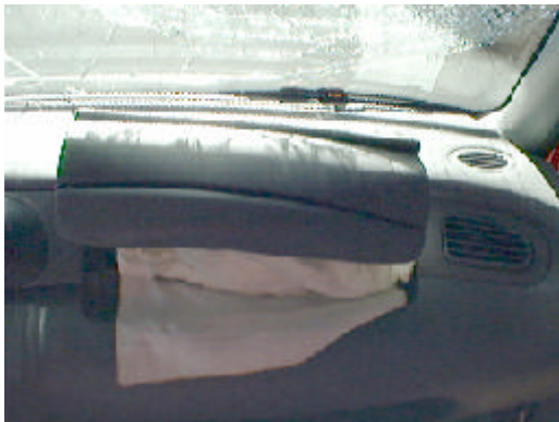
Figure 10 - View of the front right mid mounted air bag module
