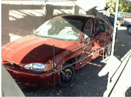
Figure 2- Left corner view of the 1998 Ford Escort showing the damage profile
