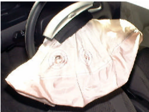
Figure 8 - View of the upper front left air bag vent ports
