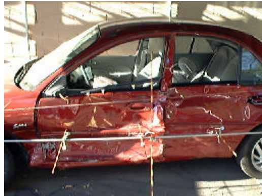
Figure 3- View showing the extent of damage at the driver door
