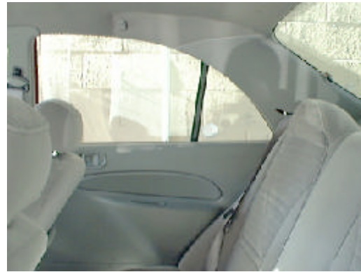
Figure 5- View of the rear seat area looking toward the right showing the relative recline position of the seat back support and the adjustment height of the head restraint
