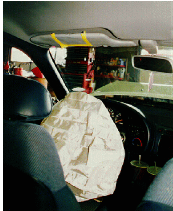
Figure 5: Case vehicle's driver seating area showing deployed air bag, contacted sun visor and rear view mirror, and noncontacted windshield (i.e., driver's portion); Note: crumpled hood visible through windshield (case photo #27)
