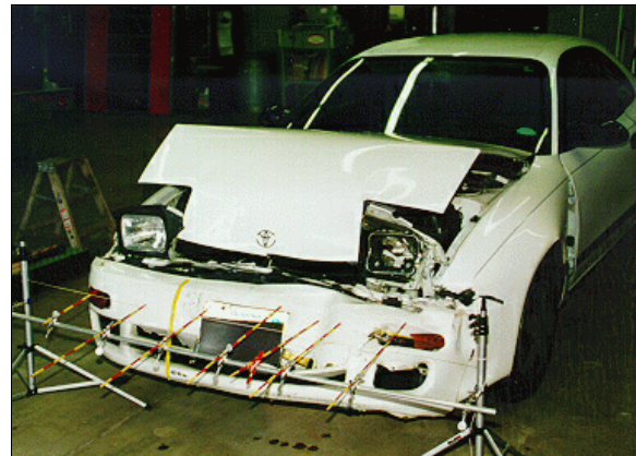
Figure 2: Case vehicle's frontal deformation with contour gauge present; Note: yellow tape indicates start of direct damage (case photo #10)
