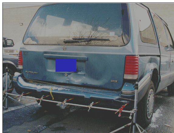
Figure 16: Deformation to vehicle #2's back with contour gauge present (case photo #55)
