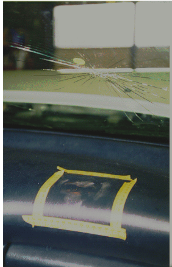
Figure 15: Close-up of starred windshield and make-up smear on top of case vehicle's right instrument panel; Note: both contacts came from front right passenger (case photo #34)
