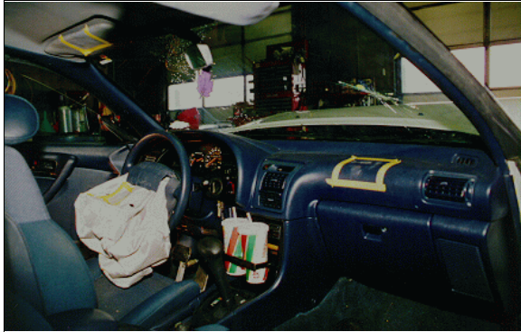
Figure 14: Case vehicle's front seating area viewed from outside right front door showing contacts (taped areas) to driver's air bag and sun visor as well as to dash and windshield on passenger's side (case photo #32)
