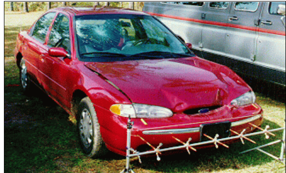
Figure 8: Case vehicle's frontal damage with contour gauge present; Note: contact to windshield's glazing on passenger side and damage on top of bumper from underride (case photo #24)
