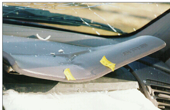
Figure 14: Close-up of blood/skin evidence on case vehicle's deformed front right air bag module's cover flap from contact with front right passenger's neck and chin (case photo #44)
