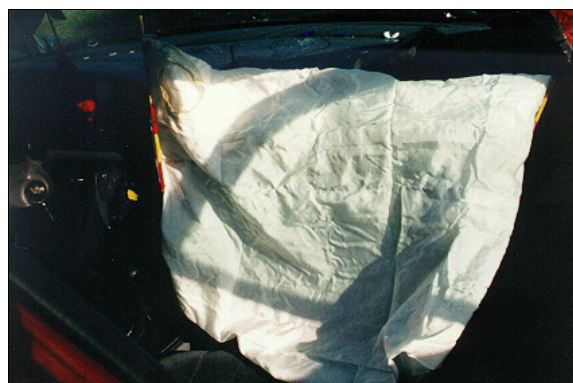
Figure 15: Front surface of case vehicle's deployed front right passenger air bag showing bloody and oily area around vent port in upper left quadrant and no other obvious evidence of contact (case photo #37)
