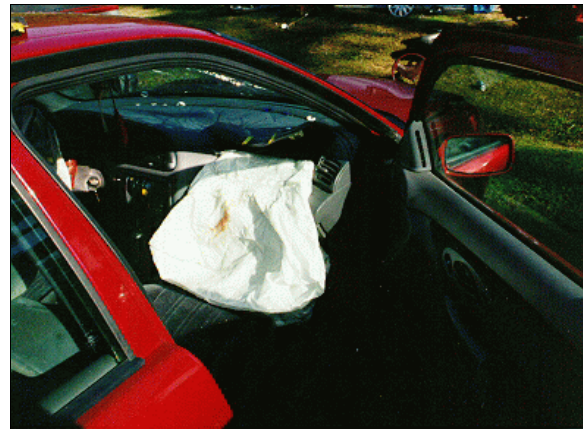
Figure 13: Case vehicle's front right seating area showing deformed front right air bag module's cover flap and blood/skin on top surface of air bag's fabric (case photo #55)
