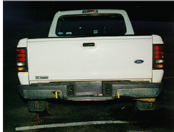
Figure 5: Minor damage to Ford pickup's back bumper; Note: yellow tape indicates direct damage to case vehicle's hood and scrapes to top of front bumper's fascia (case photo #63)
