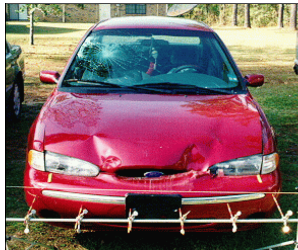
Figure 4: Case vehicle's frontal deformation from impact with Ford pickup; Note: impact to right windshield's glazing from front right passenger and imprint of pickup's back center on hood of case vehicle (case photo #08)
