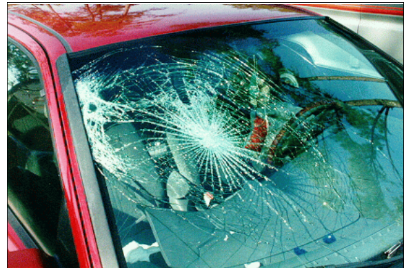
Figure 10: Close-up of case vehicle's right windshield glazing damaged from impact by front right passenger (case photo #16)
