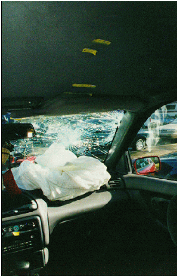
Figure 11: Vertical view of case vehicle's front right passenger seating area showing contacts to right windshield's glazing, right sun visor and header, and possibly to right roof areas (case photo #47)
