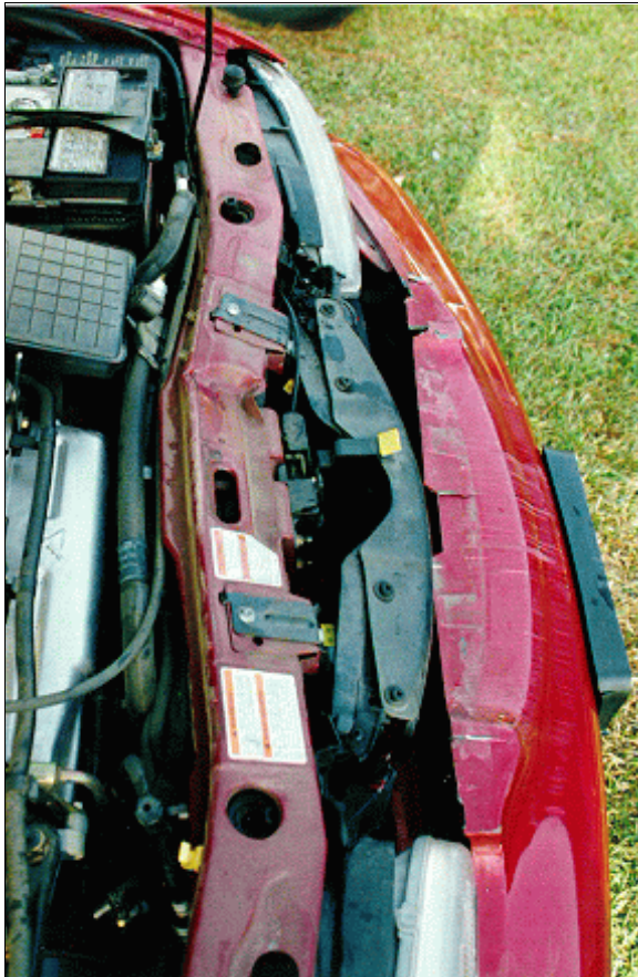
Figure 7: Elevated view from right with hood raised showing scrape on top of case vehicle's front bumper fascia; Note: air bag sensors not visible (case photo #19)
