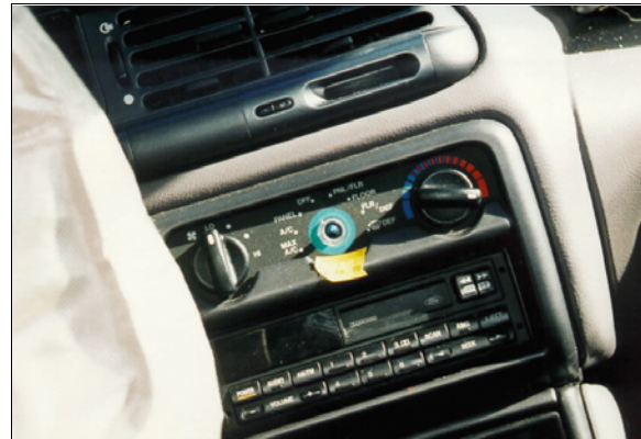
Figure 18: Case vehicle’s center instrument panel showing missing air flow knob most likely knocked off by right hand of case vehicle’s driver (case photo #36)
