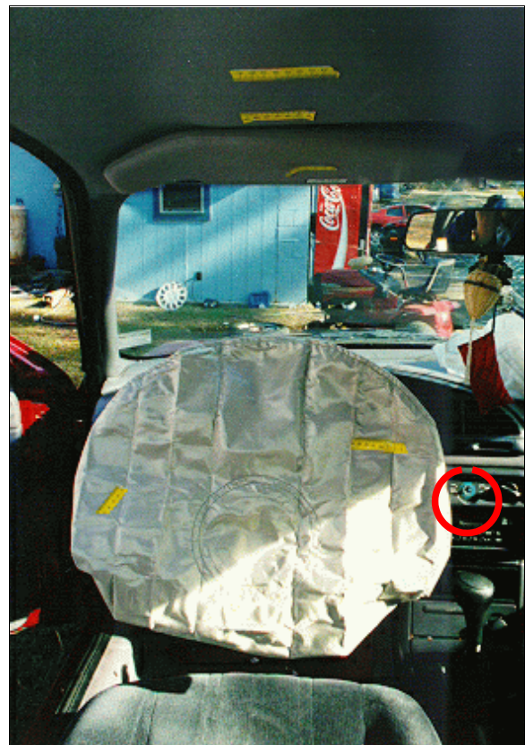
Figure 12: Vertical view of case vehicle's driver seating area showing contact evidence on air bag's fabric, center instrument panel (highlighted), and possibly to roof (case photo #31)
