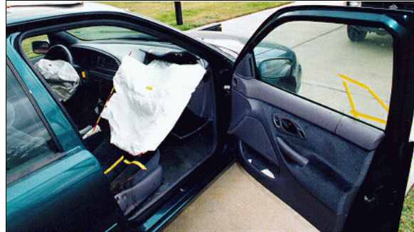
Figure 11: Interior surface of case vehicle's right front door and deployed front right passenger's air bag showing occupant contact on air bag, right front glazing, and lateral surface of front right seat (case photo #43)
