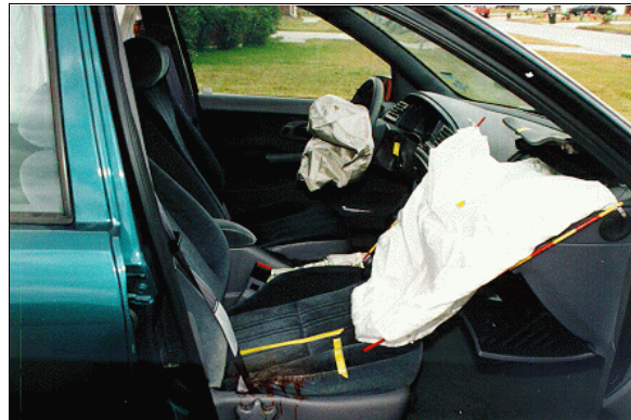
Figure 13: Case vehicle's front seating area showing deployed driver and front right passenger air bags and blood evidence on lateral side of front right seat (case photo #46)
