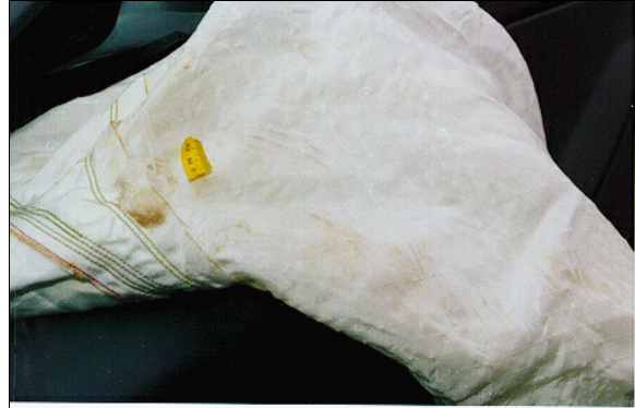
Figure 15: Underneath surface of case vehicle's deployed front right passenger air bag showing driver contact area near snag which occurred during air bag's deployment (case photo #33)
