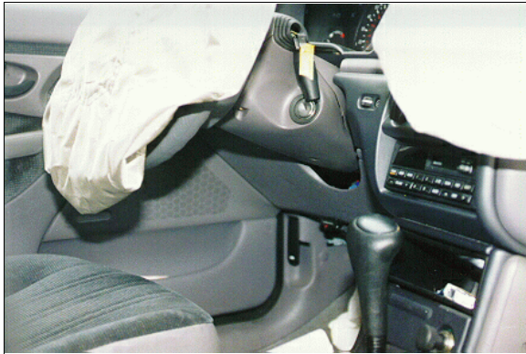
Figure 7: Case vehicle's steering column showing deployed driver air bag and broken windshield wiper lever (case photo #25)
