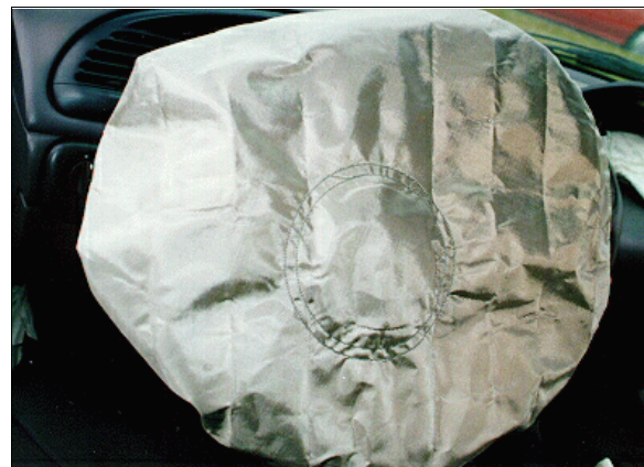
Figure 14: Case vehicle's deployed driver air bag showing no visible evidence of contact (case photo #22)
