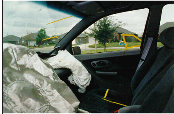
Figure 8: Case vehicle's front seating area showing deployed front air bags and driver's travel path within interior; Note: sequentially driver struck and deposited evidence on the front right passenger air bag module's cover flap, air bag, front right sun visor, and right front glazing (case photo #28)
