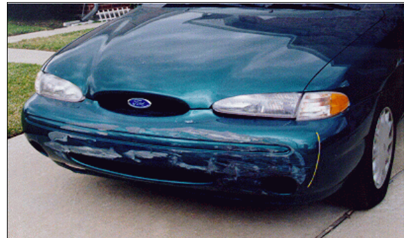
Figure 4: End swipe damage to case vehicle's front bumper fascia from concrete median barrier viewed from left of front (case photo #05)
