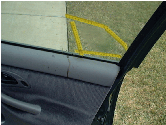
Figure 12: Case vehicle's right front door glazing showing oil and blood smear from contact by driver's head (case photo #50)
