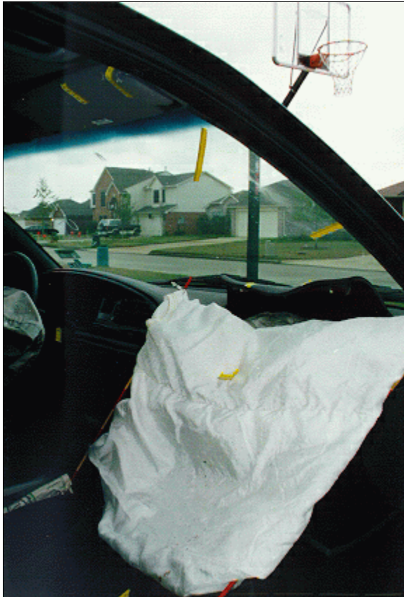
Figure 9: Vertical view of case vehicle's deployed front right passenger air bag showing evidence of driver contact to front surface of air bag, front right sun visor; and spray on the right windshield (case photo #40)
