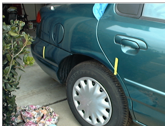
Figure 3: Sideswipe damage to case vehicle's right quarter panel above the right rear wheel well; Note: contact resulted from initial impact with concrete longitudinal barrier (case photo #16)
