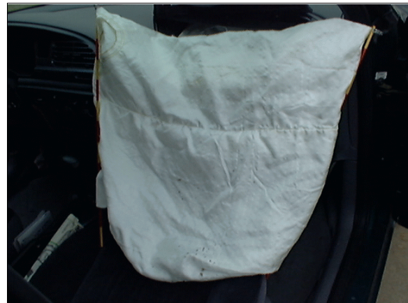
Figure 19: Case vehicle's deployed front right air bag showing evidence of occupant contact to lower right quadrant (case photo #39)
