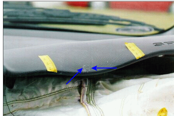
Figure 18: Close-up of deformation and teeth marks (arrow) on case vehicle front right passenger air bag module's cover flap from contact with face of case vehicle's driver (case photo #37)
