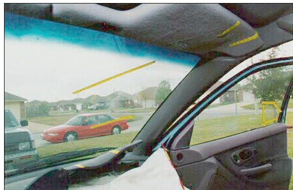
Figure 17: Case vehicle's front right seating area showing driver's direction of movement and contacts to air bag module's cover flap, sun visor, and right front door glazing; Note: spray on right windshield (case photo #30)
