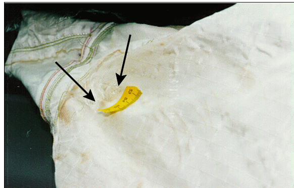
Figure 16: Close-up of snag on underneath surface of case vehicle's deployed front right passenger air bag; Note: snag (arrows) near area of skin, oil, and fluid stains from contact by driver (case photo #34)
