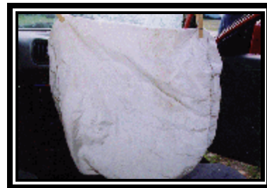
Figure 8. Tissue and vinyl transfers on the face of the front right air bag.
