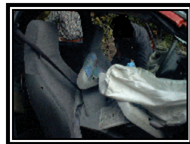
Figure 12. Excursion of the front right air bag into the CSS.
