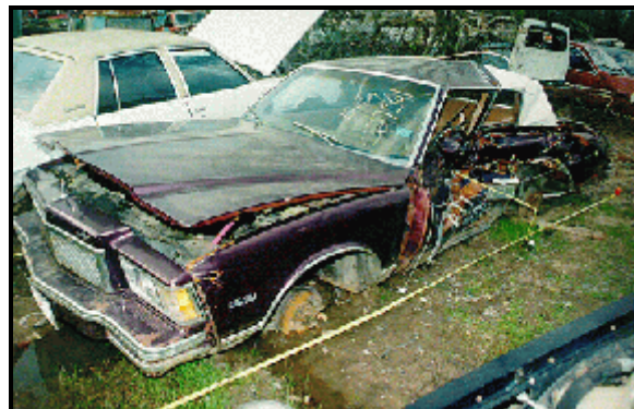
Figure 4: Vehicle #2's left-side damage; Note: direct contact to "D" pillar and "C" pillar (case photo #13)
