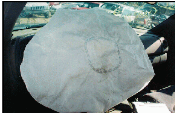
Figure 10: Case vehicle's deployed driver air bag; Note: air bag module had been removed post-crash and thrown into cargo area (case photo #40)
