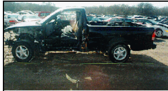
Figure 7: Case vehicle's left-side damage from impact (2nd event) with vehicle #3 (case photo #17)
