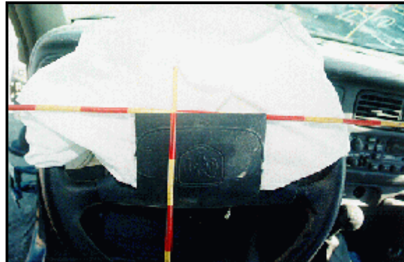
Figure 9: Close-up of case vehicle driver air bag module's cover flap; Note: steering wheel is rotated 180 degrees (case photo #45)
