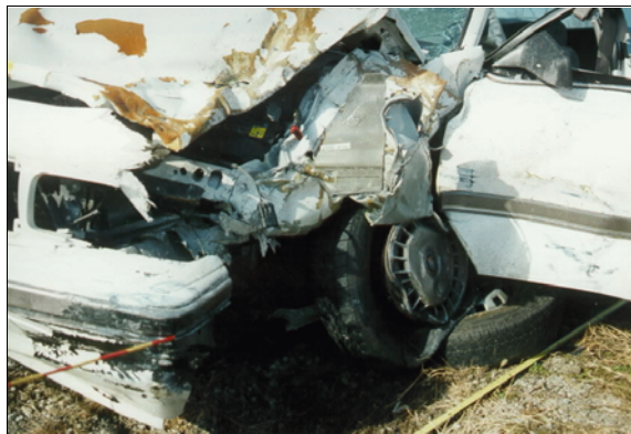
Figure 8: Close-up of case vehicle's corner impact showing damage to left front wheel assembly (case photo #14)
