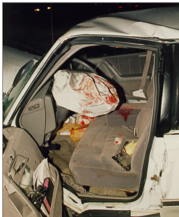
Figure 13: On-scene close-up of case vehicle's front seating area showing driver's deployed, bloodied, air bag and blood evidence on center arm rest (case photo #49)
