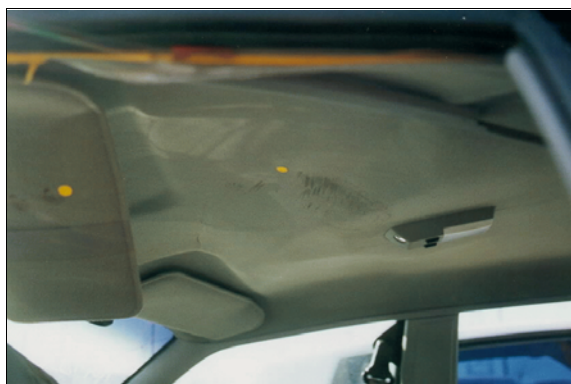
Figure 10: Sun visor and roof area on case vehicle's driver side showing contact evidence on sun visor from driver's face and roof from driver's scalp (case photo #28)
