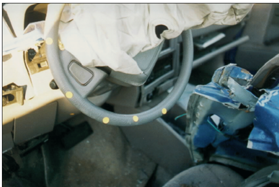
Figure 14: Contacts (i.e., scratches) along right side of Plymouth's steering wheel; Note: top of steering wheel has been rotated approximately 60 degrees clockwise in photo (case photo #53)
