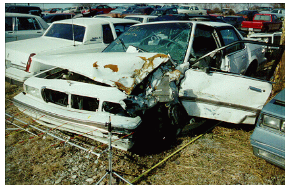
Figure 4: Case vehicle’s frontal damage viewed from left of front; Note: direct damage to left front door and induced damage to left “A”-pillar (case photo #13)
