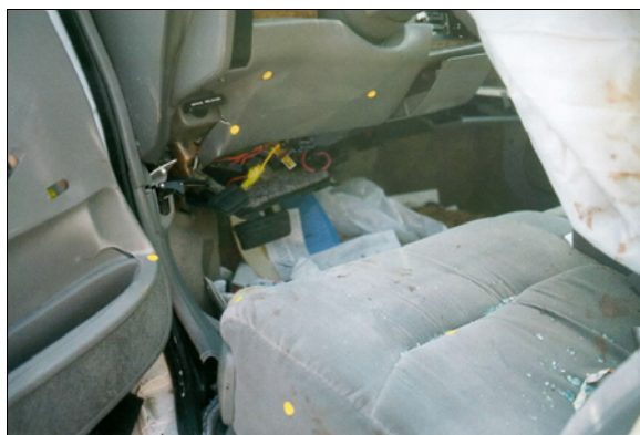
Figure 9: Contact evidence on case vehicle's driver knee bolster and left instrument panel; Note: blood splatter on driver's seat and interior surface of driver's door (case photo #25)
