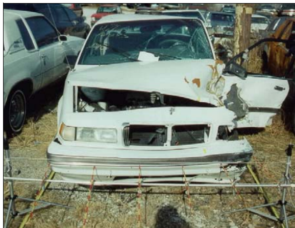
Figure 3: Case vehicle’s front left damage with contour gauge present (case photo #11)
