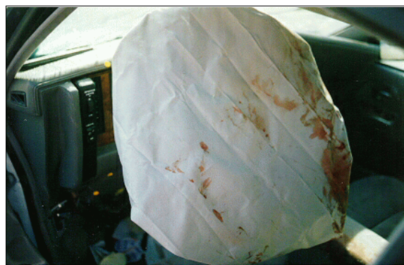
Figure 12: Case vehicle's deployed driver air bag showing evidence (i.e., blood) of contact (case photo #34)
