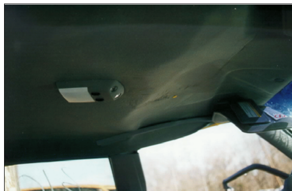
Figure 11: Sun visor on case vehicle's driver side showing deformation from impact by driver's face (case photo #33)
