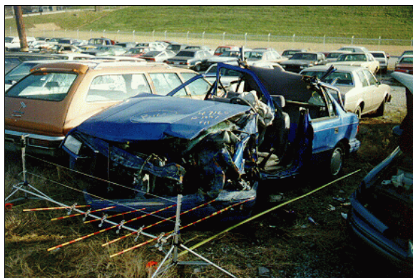
Figure 5: Plymouth's frontal damage viewed from left of front; Note: left front door and both left "A" and "B"-pillars were severed by an extrication tool (case photo #38)
