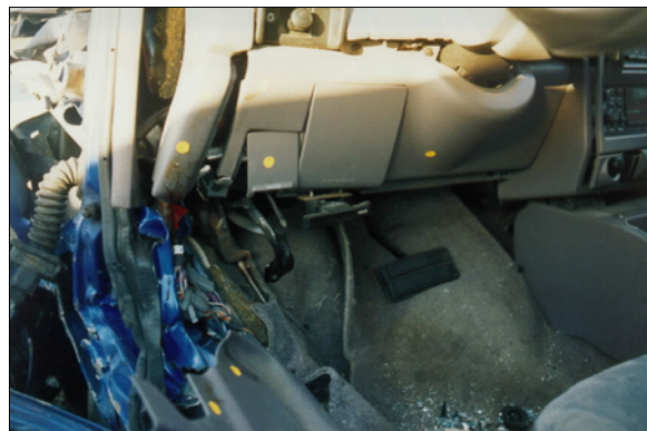
Figure 15: Contact evidence on Plymouth's driver knee bolster and left instrument panel; Note: contacts to interior surface of driver's door (case photo #52)
