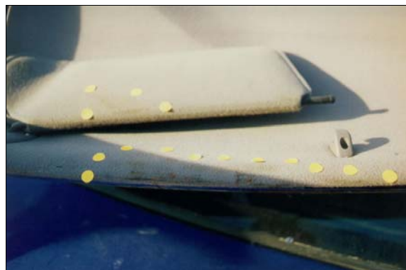
Figure 17: Close-up of contact evidence found on Plymouth's driver sun visor and left windshield header (case photo #56)
