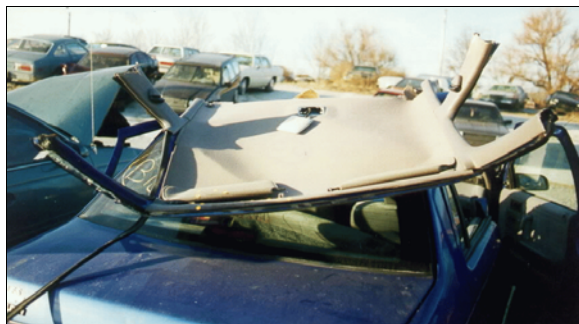
Figure 16: Interior surface of Plymouth's roof, peeled back during extrication, showing contact evidence to driver's sun visor and left windshield header (case photo #55)
