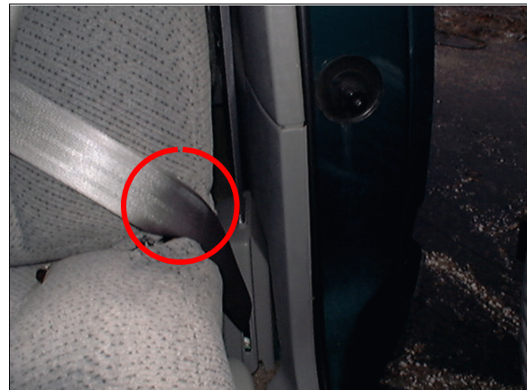
Figure 11: Case vehicle's driver seat belt showing heat abrasion (highlighted) on lap belt portion of webbing (case photo #19)
