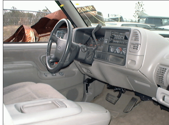
Figure 6: Case vehicle's driver seating area showing non-deployed driver air bag (case photo #13)
