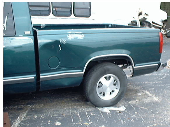
Figure 5: Side slap damage on left side of case vehicle's pickup bed (case photo #07)
