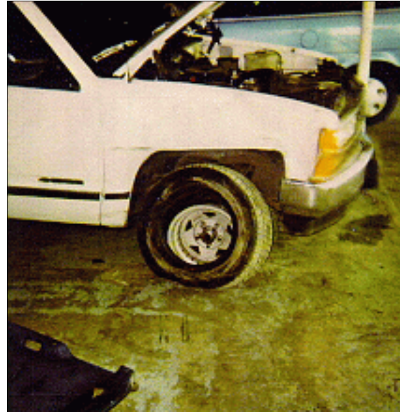
Figure 4: Insurance photo of damage to 1992 Chevrolet pickup's right fender and right front wheel assembly (case photo #25)
