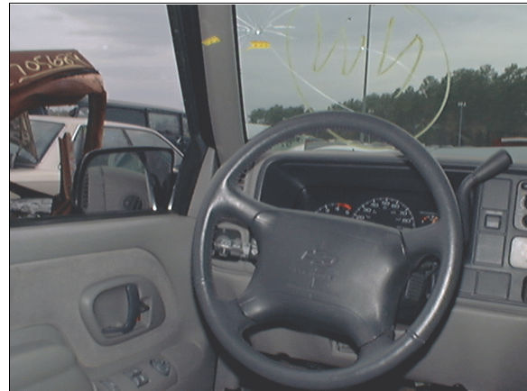
Figure 10: Case vehicle's non-deployed driver air bag; Note: evidence of driver contact (yellow tape) on left side of windshield's glazing and left "A"-pillar (case photo #22)
