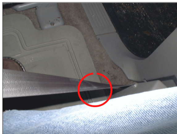
Figure 13: Overhead view of case vehicle’s front right passenger safety belt showing heat abrasion (highlighted) on lap belt portion of webbing (case photo #21)
