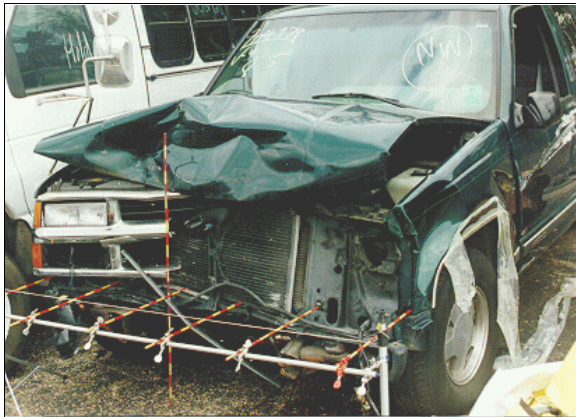
Figure 3: Case vehicle's frontal deformation viewed from left of front with contour gauge present (case photo #06)
