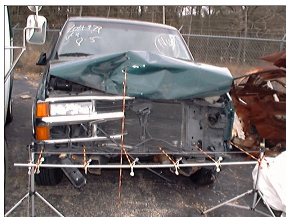
Figure 2: Case vehicle's frontal deformation with contour gauge present; Note: vertical rod approximates location where 1992 pickup's right front corner penetrated case vehicle's hood (case photo #03)
