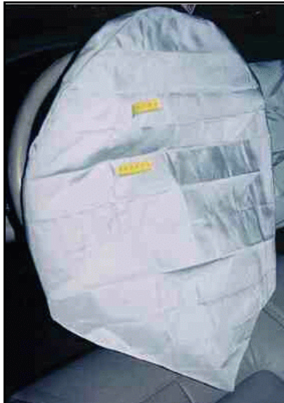
Figure 8: Case vehicle's driver air bag with contact evidence marked (case photo #24)
