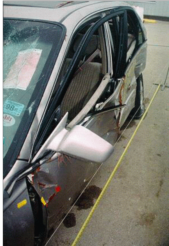
Figure 3: Case vehicle's damaged left front door from first impact; Note: contact near forward seam of door panel and on "A" pillar (case photo #25)
