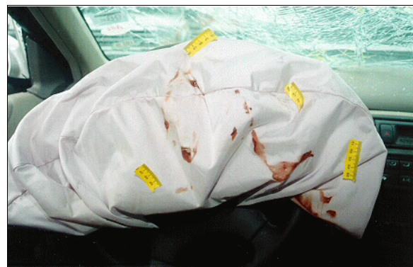
Figure 10: Case vehicle's driver air bag; Note: blood stains on bottom, back side of fabric (case photo #64)
