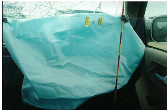
Figure 11: Case vehicle's front right passenger air bag; Note: three blood splatters on top right quadrant of the fabric (case photo #67)
