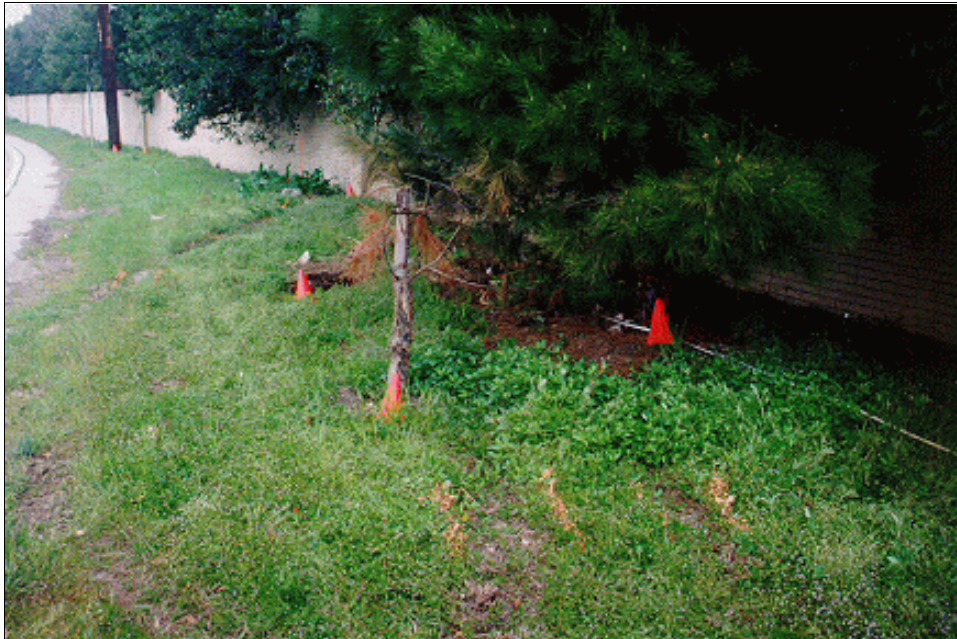
Figure 15: Case vehicle's five impacts; Note: center cone shows impact #1, right cone shows impact #2, left cone shows impact #3, cone at wall shows #4, and utility pole was impact #5 (case photo #06)
