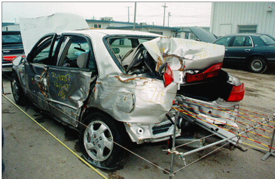
Figure 14: Case vehicle's left side damage; Note: first impact at left front door's forward seam, third impact at mid-left front door, and fourth impact goes forward from left rear corner to left front door's rear seam (case photo #28)
