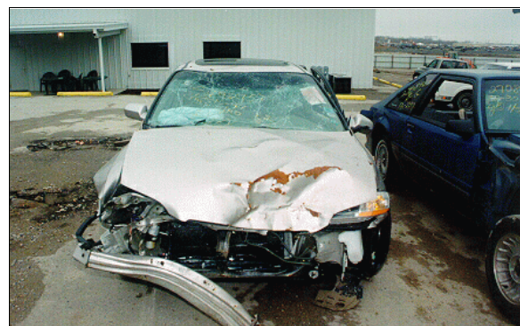
Figure 4: Case vehicle's frontal damage from the second tree (deployment) impact (case photo #18)
