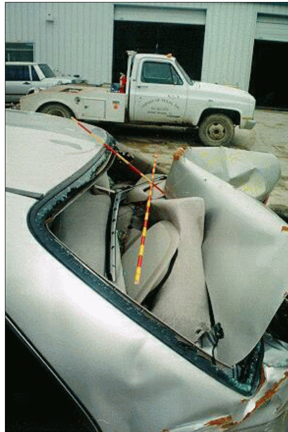
Figure 6: Case Vehicle's backlite and deck damage; Note: trunk lid intrusion into lower glazing (case photo #31)
