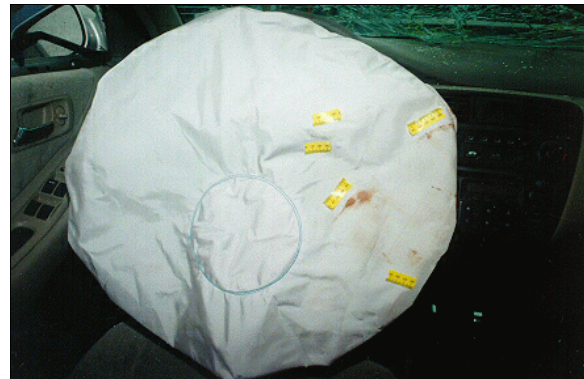
Figure 9: Case vehicle's driver air bag; Note: blood stains and scuffs to right third of fabric (case photo #58)
