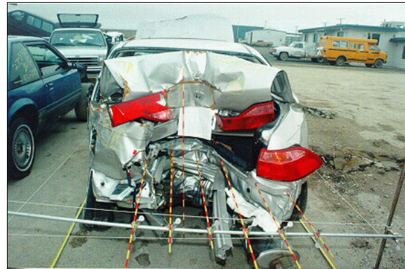
Figure 5: Case vehicle's back damage from utility pole (fifth impact; Note: pole was highest Delta V impact (case photo #32)
