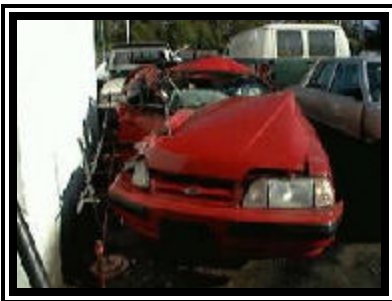
Figure 4. Right side surface damage to the 1991 Ford Mustang LX.
