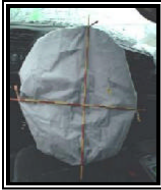
Figure 6. 1998 Chevrolet S-10 Blazer redesigned driver air bag.
