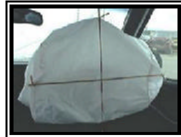
Figure 8. 1998 Chevrolet S-10 Blazer redesigned passenger air bag.
