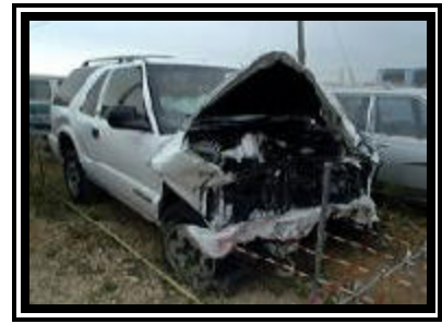
Figure 3. Frontal damage to the 1998 Chevrolet S-10 Blazer.
