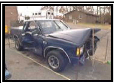
Figure 4. Frontal damage to the 1988 Chevrolet pickup truck.
