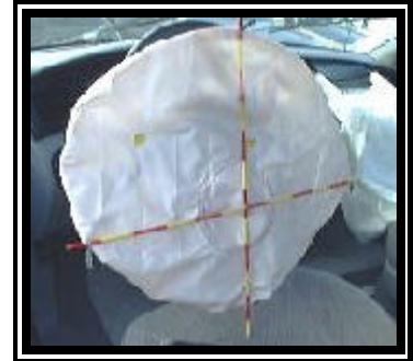
Figure 5. 1998 Ford Windstar redesigned driver air bag.
