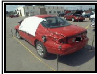
Figure 7. Left side and top rollover damage.
