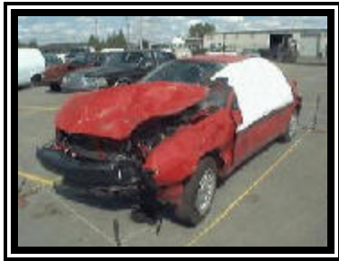
Figure 6. Front left damage to the 1998 Ford Escort ZX2.
